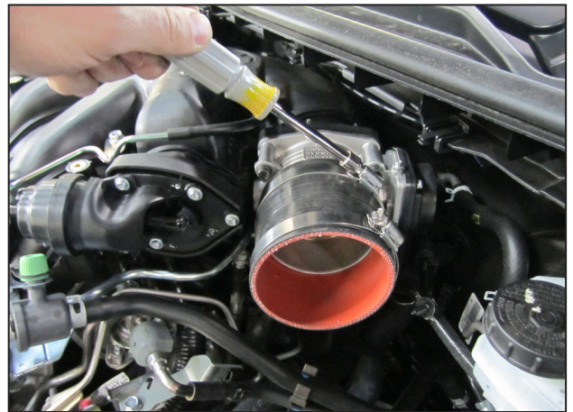
c. Tighten the #52 hose clamp on the throttle body end.
