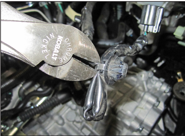
u. Cut and remove the clip from the MAF sensor harness as shown. NOTE: Use caution and DO NOT cut the MAF sensor wire harness.
