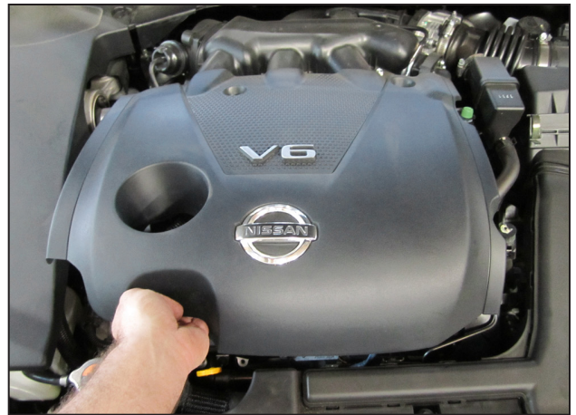
b. Lift up on the bottom of the engine cover and remove from the vehicle.
