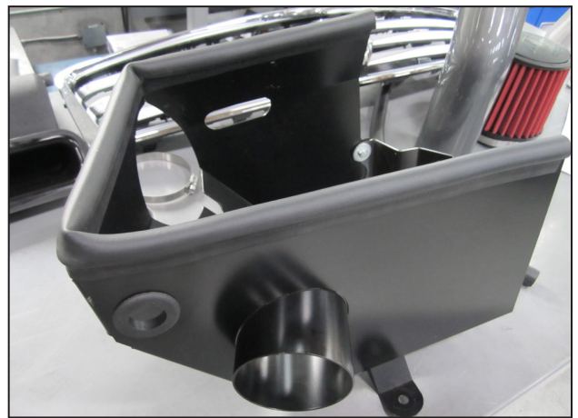
k. Install the rubber edge trim (8-4030) onto the top edge of the heat shield.
