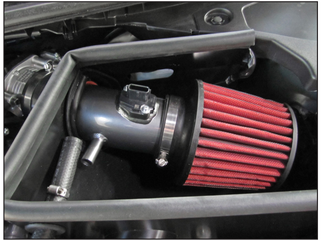
ag. Insert the intake pipe assembly into the heat shield as shown.
