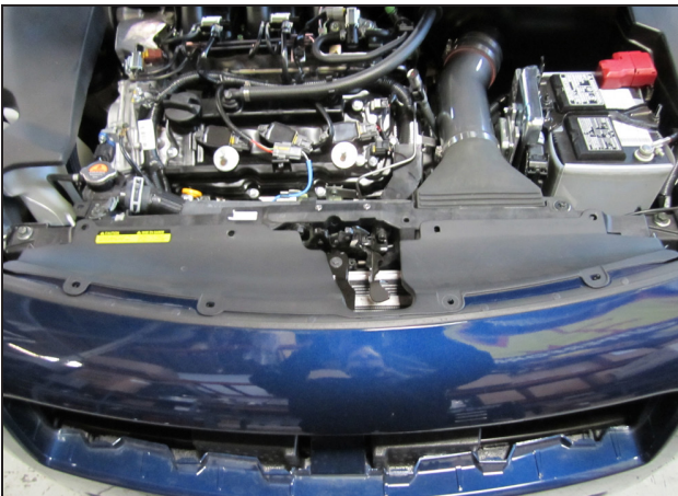
an. Reinstall the radiator shroud.
