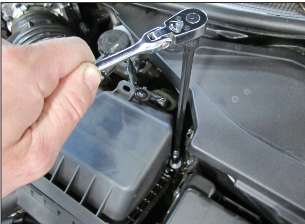
i. Remove the 10mm bolt that secures the lower air box in place.
