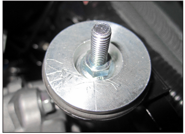
g. Use the provided M6 nuts (444.460.04) to keep the assembly together.
