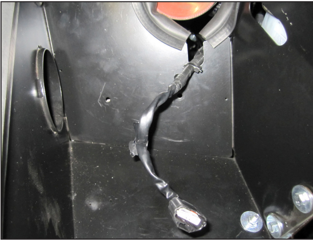
af. Feed the MAF sensor wire harness into the inside area of the heat shield as shown.
