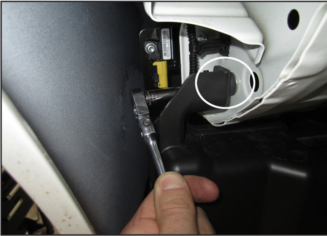
aa. Remove the lower 10mm bolt securing the resonator tube.
