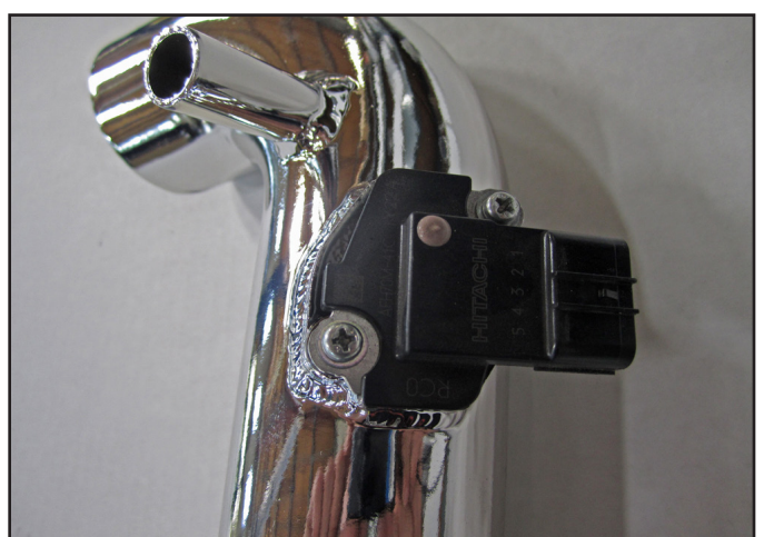
e. Install the mass air sensor into the upper intake tube.
