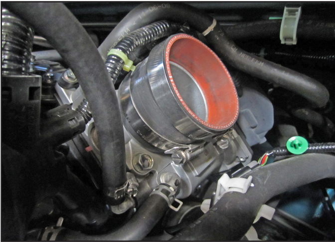
f. Install the coupler and two #40 hose clamps onto the throttle body.
