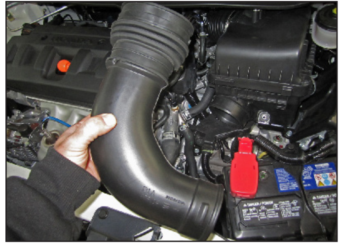
d. Pull the air duct out of the vehicle's engine compartment.
