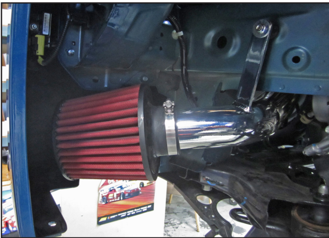
n. Install the AEM® Air Filter onto the lower intake tube and tighten the #44 hose clamp.
