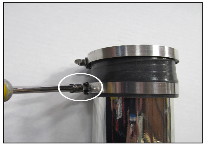
i. Tighten the hose clamp on the upper intake tube.
