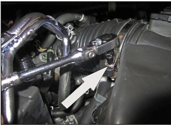
e. Loosen the hose clamp at the air box.
