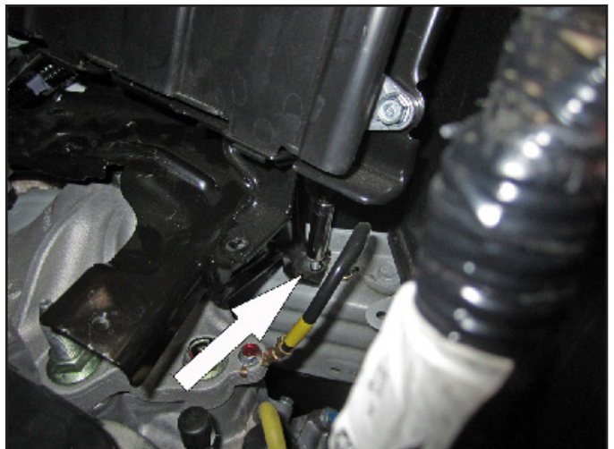
l. Remove the lower 10mm bracket bolt.
