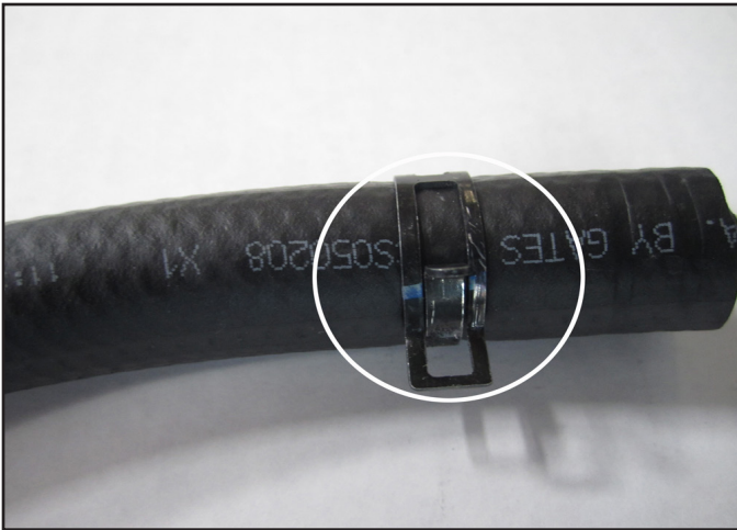
r. Install the OEM PCV clip onto the 5/8" hose.
