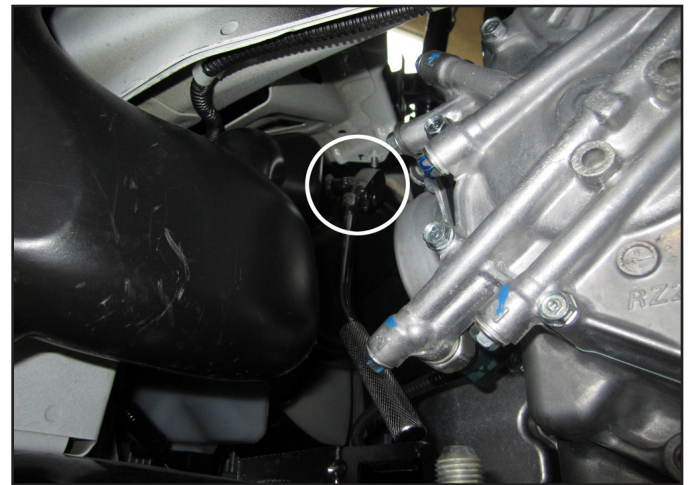
z. Remove the upper 10mm bolt securing the resonator tube.
