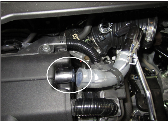
s. Release the clip on the valve cover for the PCV hose, then remove the hose from the valve cover.
