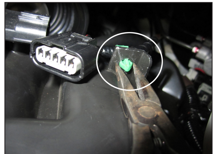
h. Release the mass air sensor clip on the air box.
