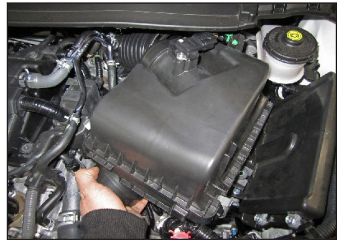
f. Pull up firmly to dislodge the air box from the mounting grommets, then pull it forward.
