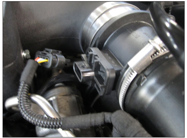
r. Re-install the MAF housing into the turbo inlet tube and then into the reinforced hose. The flange should face the hose. Orient the MAF sensor as shown.
