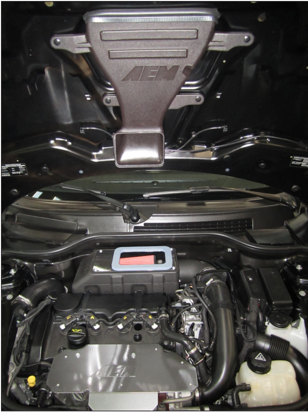
k. Complete AEM® 21-721C Cold Air Intake installed. NOTE: The top lip of the scoop inlet will be visible through the hood opening. This small gap allows cooling air flow over the scoop and venting after hot shutdown.
