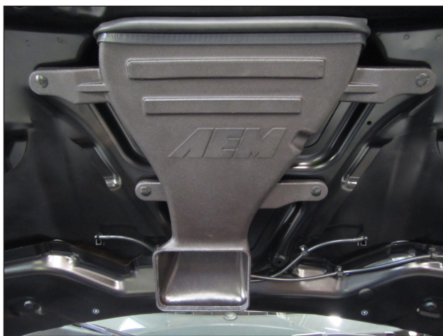
j. Mount the AEM® cold air intake scoop (C) onto the mounting holes using the 4 plastic push rivets (L). Make sure the rivets are fully seated. Tuck the edge trim as needed to complete the seal around the air inlet.
