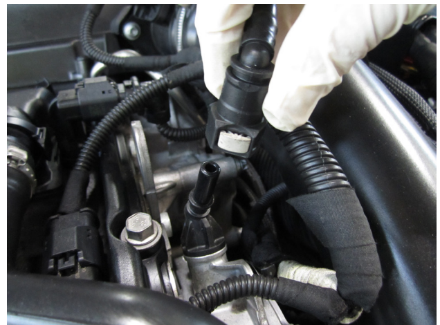
d. Disconnect the vacuum line port.
