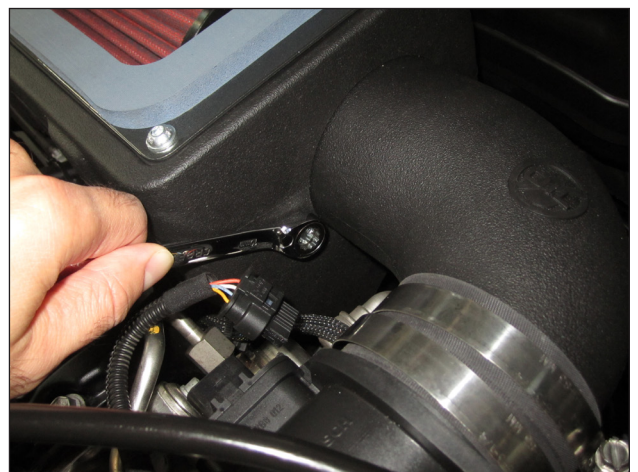
v. Next, fully tighten the 2 bolts that were installed in step 3d to lock the intake elbow in place. Re-connect MAF Sensor.
