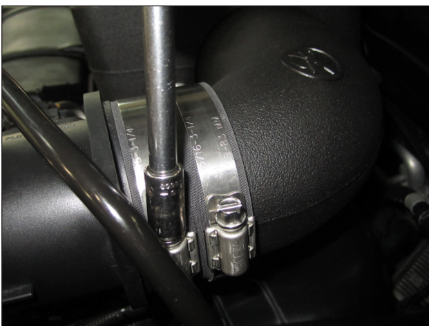
u. Next, straighten the two #44 hose clamps as shown and then fully tighten.
