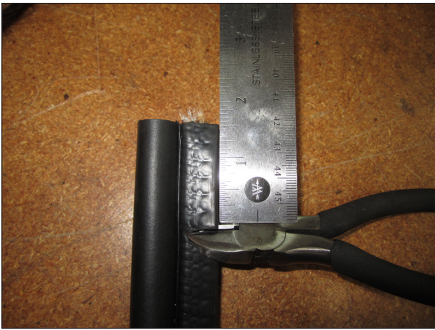
e. Cut slits in the edge trim seal (J) on one side of the clamp using a razor or wire cutters about 1-1/2" [~38mm] from each end. Cut through the rubber clamp only. Avoid cutting the metal clips inside the clamp.
