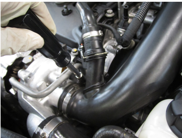
c. Loosen the hose clamp at the turbo inlet.
