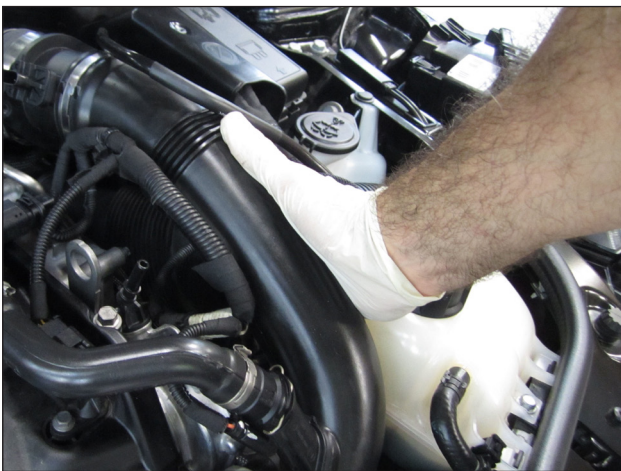
s. Push down on the stock turbo inlet tube to rotate it down back to its original position.
