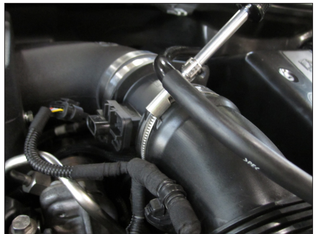
t. First, tighten the hose clamp between the MAF housing and the stock turbo inlet tube.
