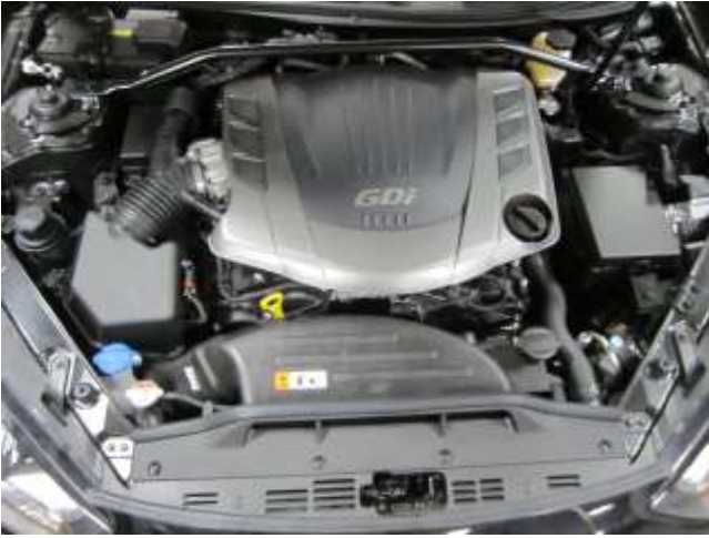
STOCK INTAKE INSTALLED
