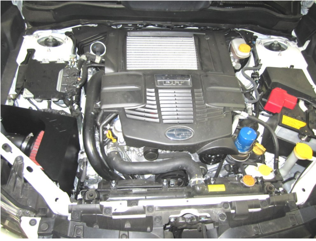
k. AEM intake system installed.
