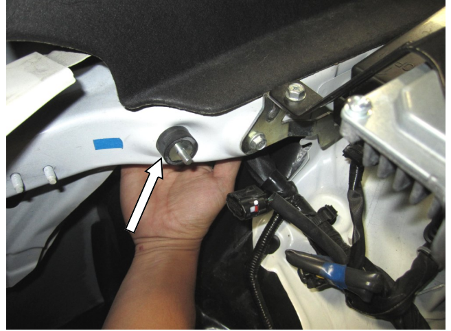
b. Install the supplied rubber mount(07027) onto the fender frame and fasten from behind using the supplied washer(08160) and nut(444.460.04).
