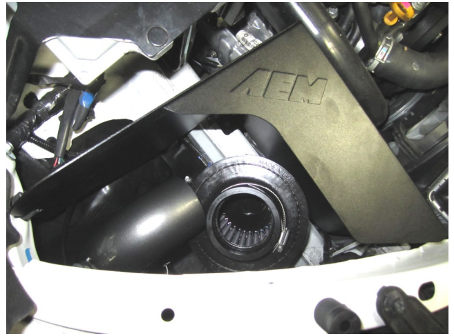
f. Place filter and hose clamp near the AEM tube as shown and set heat shield(20-8541) into place.
