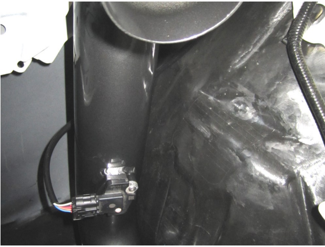
e. Connect the extension harness(8-197-1) to the stock harness, around the tube, and plug into the MAF sensor.
