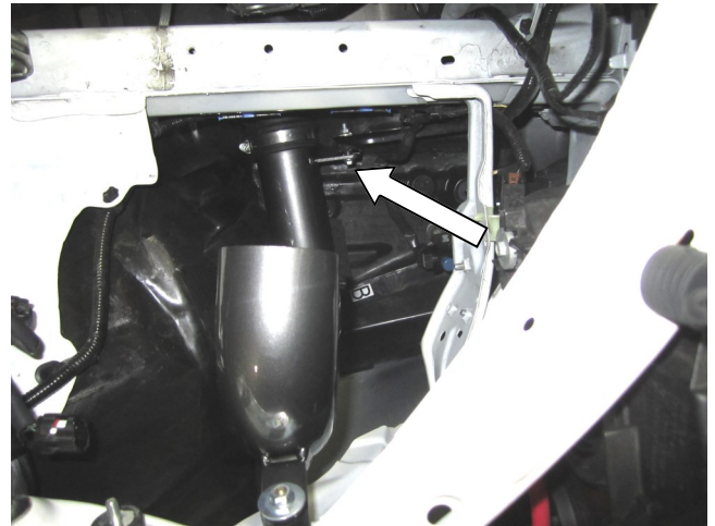
d. Install the AEM tube into the stock lower bellow coupler. Align the lower bracket to the stock rubber mount and fasten with the original nut from step 2f. Fasten upper bracket to the rubber mount installed in step 3c using the washer(08160) and nut(444.460.04) provided. Check for clearance around tube and fasten the stock hose clamp to secure the bellow coupler to the tube.
