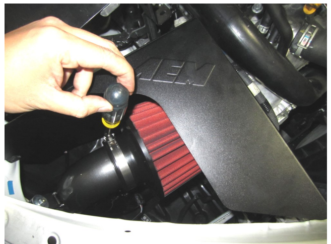
j. Carefully slide air filter onto the AEM tube. Check for clearance around the filter and fasten hose clamp(9448).
