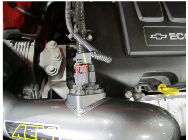
l. Reconnect the harness to the sensor that was removed in step 2a.
