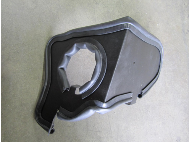
a. Install all 3 pieces of edge trim onto the heat shield as shown..
