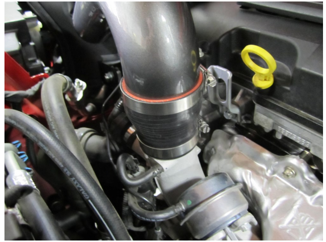
j. Install the other end of the AEM intake tube into the coupler.
