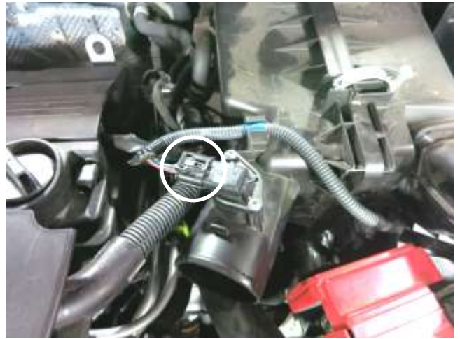
f. Unplug the electrical connector from the mass air sensor.
