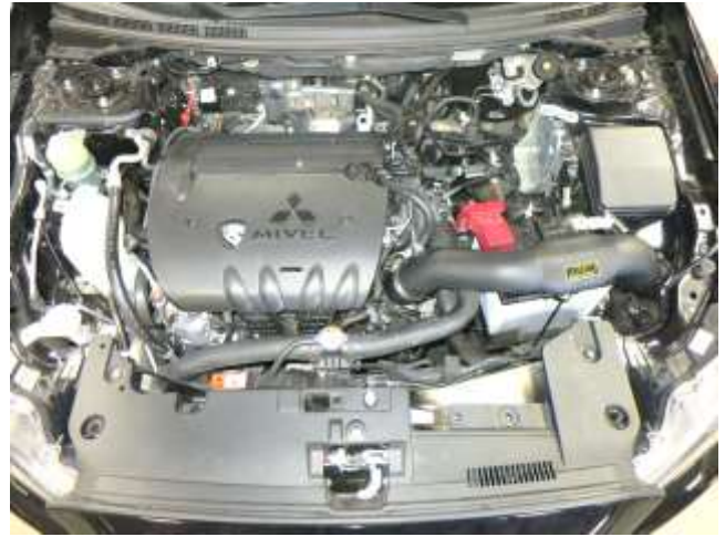
AEM INTAKE INSTALLED
