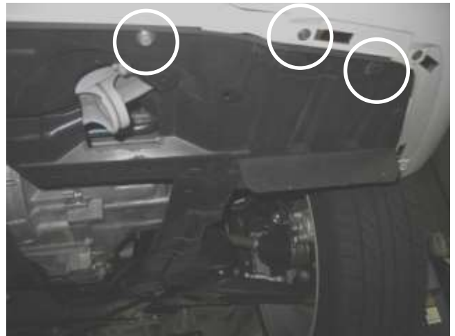
j. Raise the front of the vehicle with a jack. Refer to your owner's manual for proper jack and jack stand placement to properly support vehicle. Support your vehicle using properly rated jack stands before wheel removal or while working under the vehicle. NEVER WORK UNDER A VEHICLE WITHOUT USING JACK STANDS. Remove the plastic trim underneath the front of the vehicle on the driver side.
