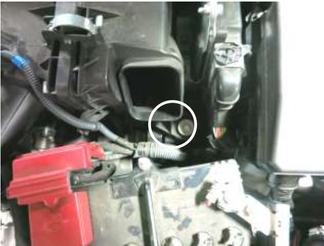
g. Remove the bolt that holds the factory air box in the engine compartment.
