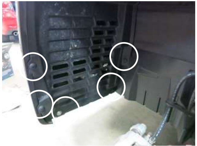
l. Remove the driver side fender well liner, it is secured to the wheel well with plastic clips and a 10mm hex bolt. This will be re-installed in step 3o.
