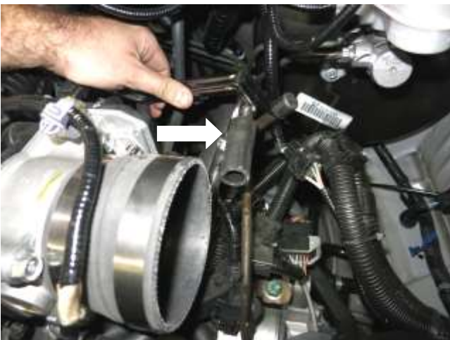
i. Install the provided vent hose onto the stock vent tube. Note: Warm soapy water may help installation.
