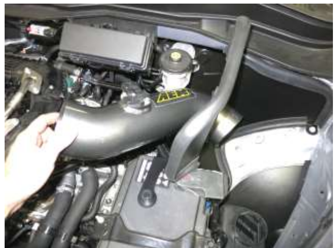
j. Install the AEM intake tube into the heatshield by inserting it as shown and maneuvering it into place, aligning it with the coupler.
