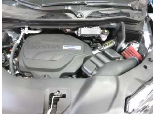
AEM INTAKE INSTALLED
