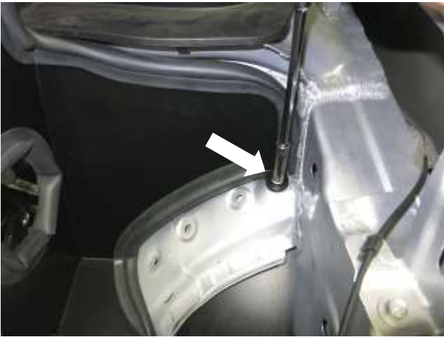
e. Using the supplied bolt, tighten heatshield mount at inner fender location ensuring the rubber washer is still in its location. Ensure other heatshield mounting hole lines up properly during tightening.
