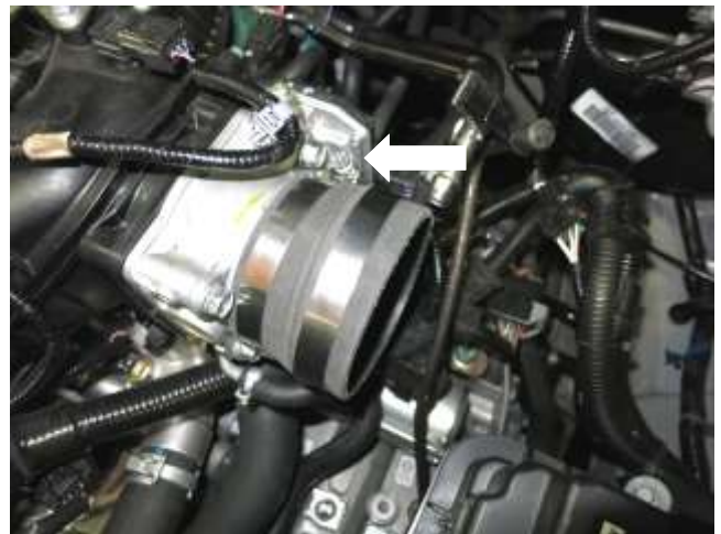
h. Install the supplied coupler and two smaller hose clamps onto the throttle body. Tighten the throttle body side coupler to 30 in-lbs at this time.
