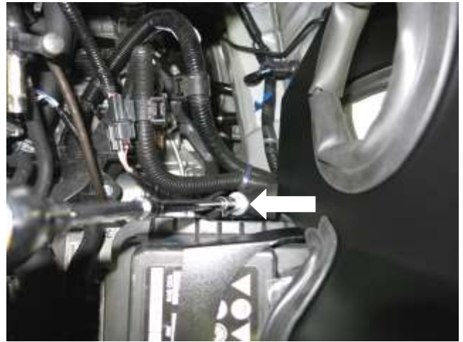
f. Using the supplied bolt and washer, tighten the heatshield mount behind the battery box.
