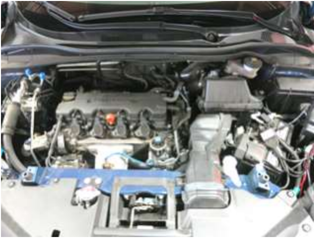
STOCK INTAKE INSTALLED
