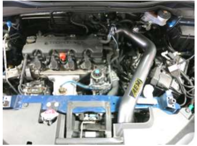
AEM INTAKE INSTALLED
