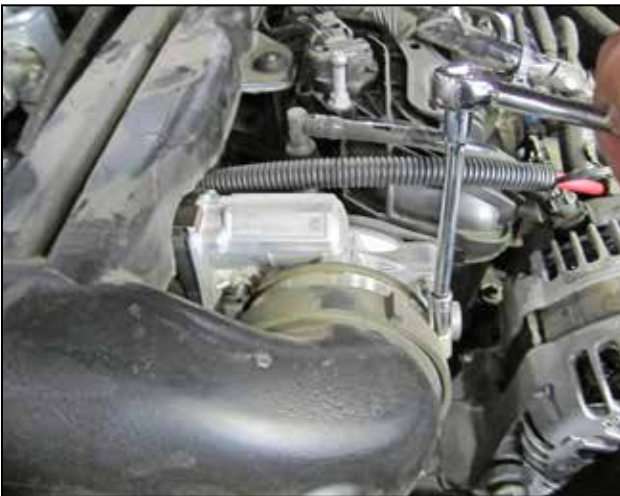
c. Loosen the hose clamp on the throttle body end of the inlet tube.
