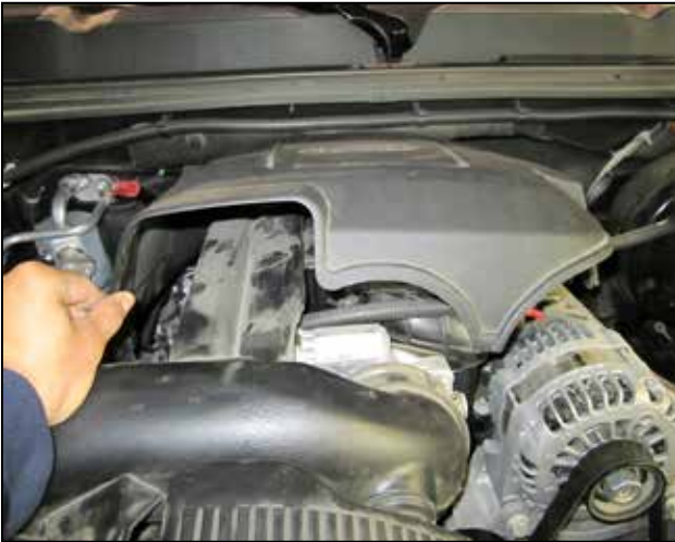
a. Remove the engine cover; lift up to release the tabs from the grommets that secure it in place.
