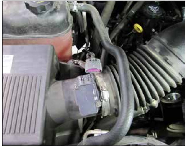
b. Unplug the MAF sensor connector from the MAF sensor.
