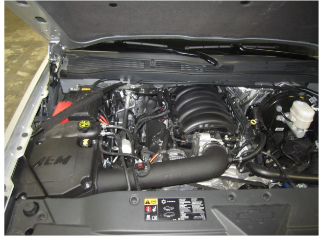
AEM intake system installed
