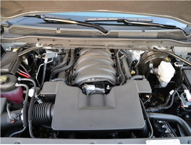
Stock intake system Installed
