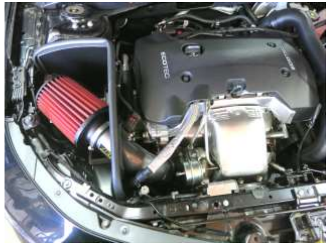
AEM INTAKE INSTALLED
