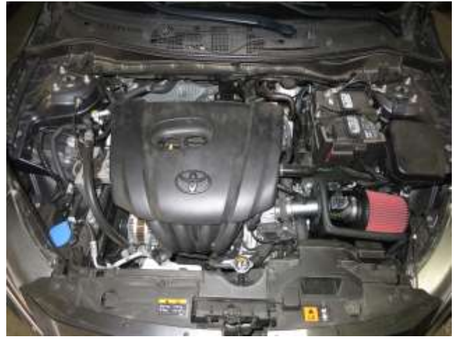
AEM INTAKE INSTALLED
