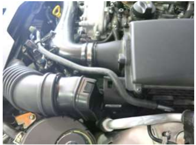
b. Pull the intake scoop from the air box and move it aside.
