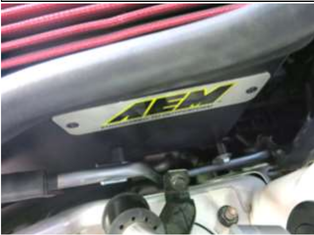
g. Angle the air box to gain as much access to the side as shown. The supplied spacers will go in between the EVAP hardline and the air box. Use the supplied M6 x 20mm bolts to fasten the hardline bracket closest to the firewall first. Then, fasten the hardline bracket towards the front of the vehicle.
