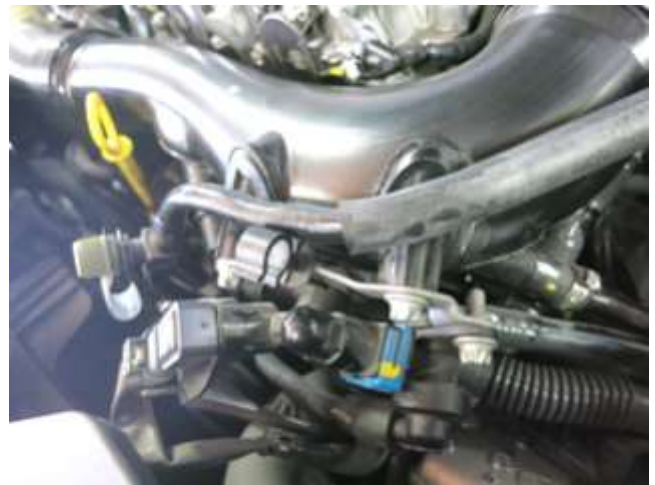
d. Remove the evaporative emissions (EVAP) hardline from the clip.
