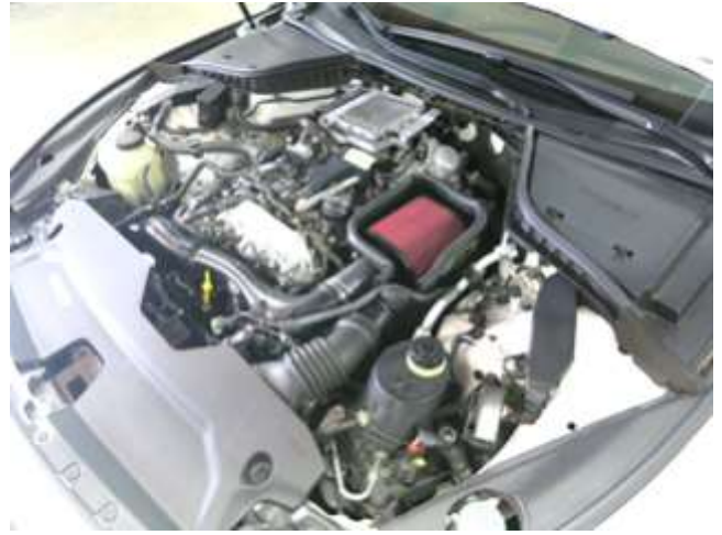
AEM INTAKE INSTALLED (ENGINE COVER REMOVED)
