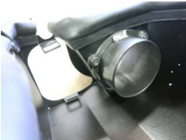
d. Make sure the flat edge on the tube flange coincides with the corresponding edge of the air box.
