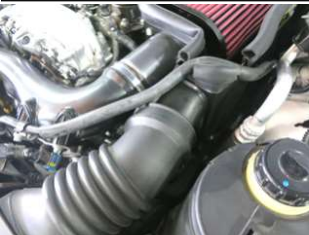
i. Insert the intake scoop into the air box. Make sure the retaining tabs on the air box lock onto the intake scoop.
