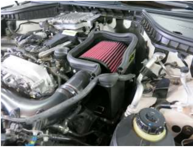
f. Place the air box assembly into the engine bay. Insert the intake tube into the turbo inlet pipe. Do not tighten the hose clamp yet and do not seat the grommets onto their posts at this time.
