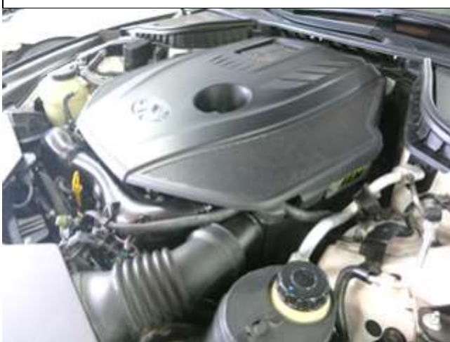
j. Reinstall the engine cover. AEM recommends you retain the use of the engine cover as the edge trim on the AEM air box is designed to seal with the engine cover to keep intake air temperatures at a minimum.
