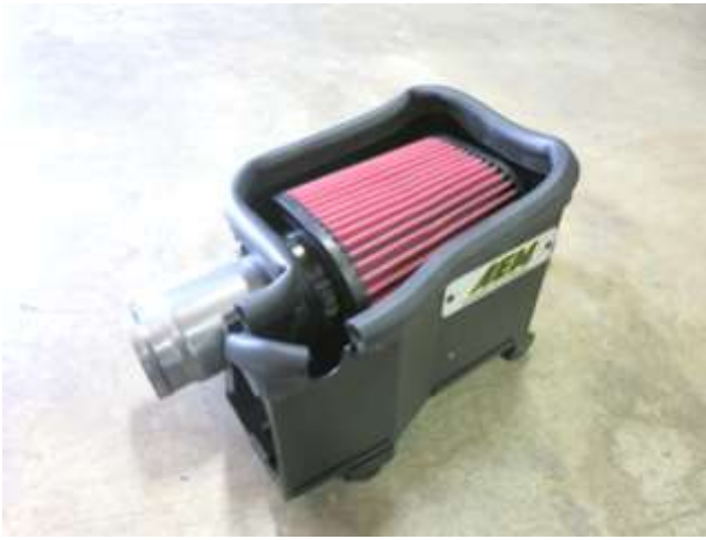
e. Install the AEM filter with hose clamp into the air box and tighten to 30 in-lbs.
