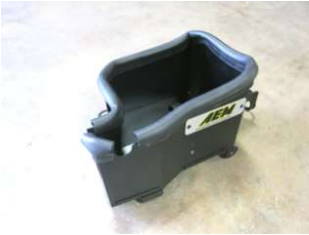
a. Line the upper edge of the AEM air box with the supplied edge trim as shown.
