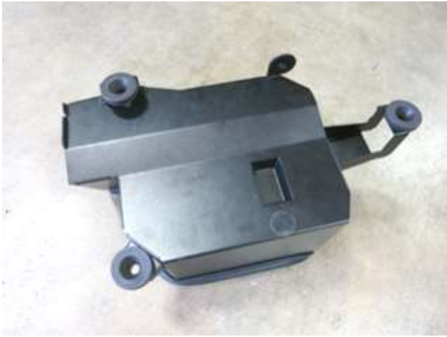
b. Install the (3) grommets removed from the factory air box onto the AEM air box as shown. Also apply the neoprene adhesive pad in the location shown.
