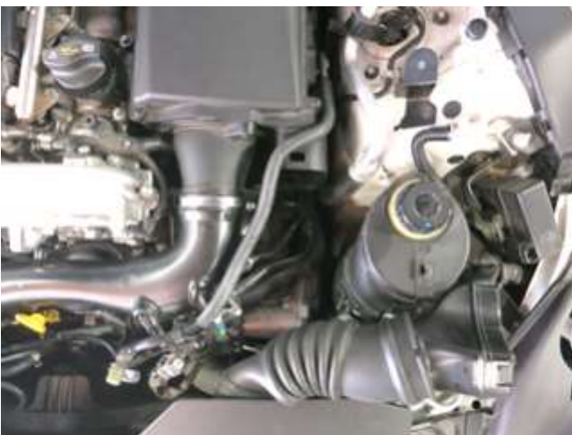
c. Loosen the hose clamp securing the air box to the turbo inlet pipe using a 7mm nut driver.
