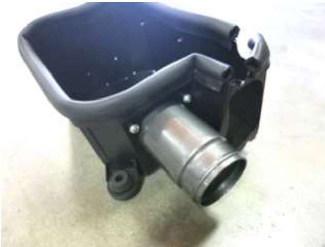
c. Install the intake tube onto the air box with the supplied (3) M6 button head bolts and (3) split lock washers.
