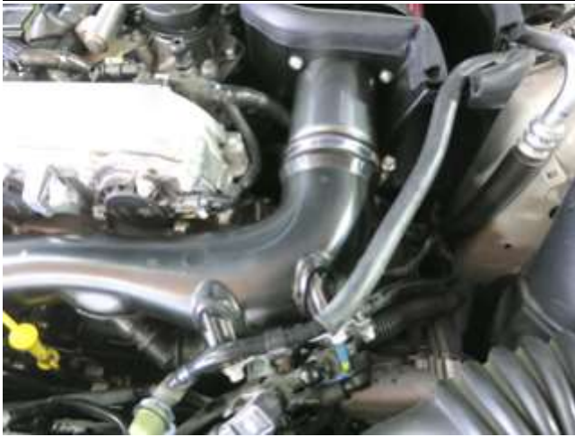
h. Push down on the air box to fully seat the grommets onto their respective posts. Tighten the hose clamp and reattach the EVAP hardline to the clip.
