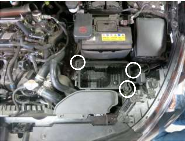
g. Remove the (3) bolts that secure the lower air box housing with a 10mm socket and ratchet.
