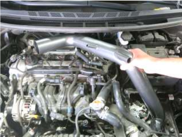
c. Install the AEM intake tube by dropping the filter end inside the frame rail first, then swing the turbo inlet side in towards the fire wall.
