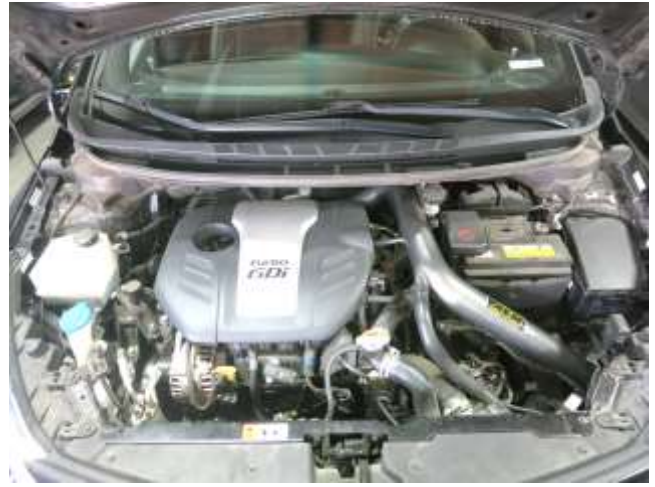
AEM INTAKE INSTALLED
