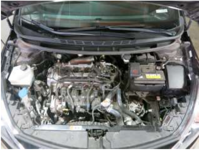
h. Lift and remove the lower air box housing and scoop.. AEM recommends that you do not discard the factory intake system.
