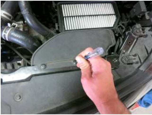
f. Remove the 2 clips holding the air scoop with a screwdriver by depressing the center pin. Do not discard the clips.
