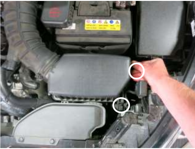
e. Detach the 2 latches from the air box lid from the lower air box housing and remove air box lid and intake hose.
