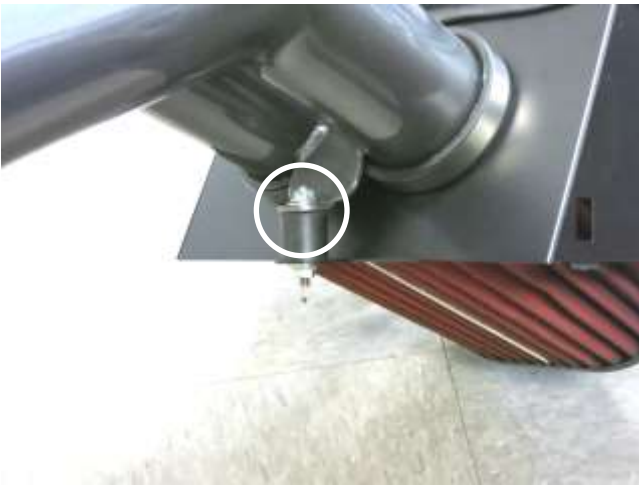
g. Install the provided nut and washer onto the AEM intake tube bracket, then tighten both sides.
