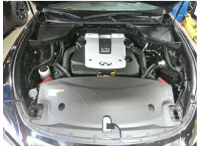
AEM INTAKE INSTALLED
