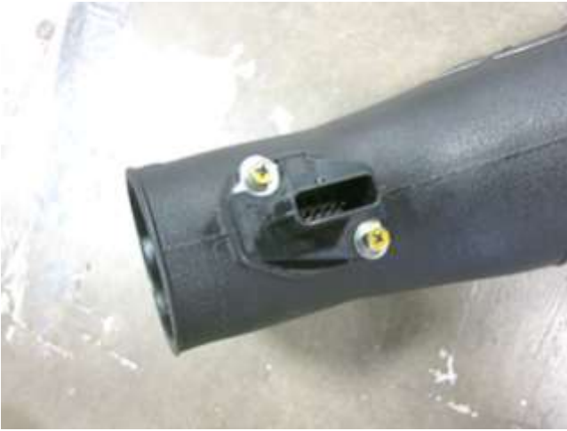
a. Install the MAF sensors into both AEM intake tubes.
