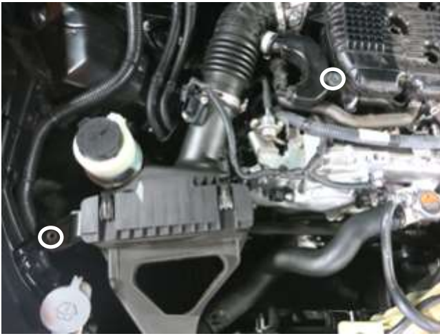
e. Remove the [2] M6 bolts in the locations shown above.
