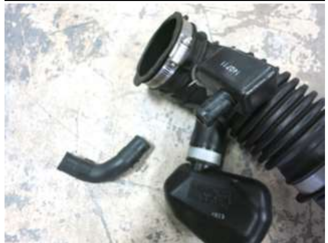
j. Pull the breather hose from the intake tube (driver side pictured).
