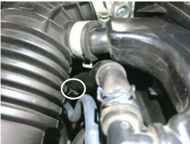
g. Use pliers to release the spring clamp shown above (passenger side pictured).
