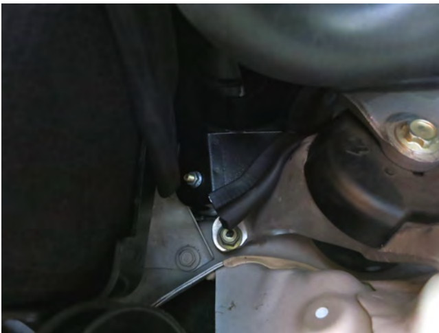
i. Fasten the heatshield base to the lower rubber mount with the provided nut.
