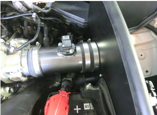
g. Lower the heat shield assembly into the engine bay and connect the intake tube to the filter adapter. Then, connect the factory air scoop to the heatshield.
