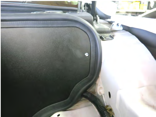
h. Fasten the heatshield at the shock tower with the provided bolt.
