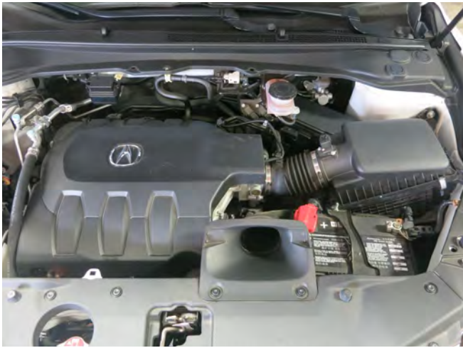
STOCK INTAKE INSTALLED
