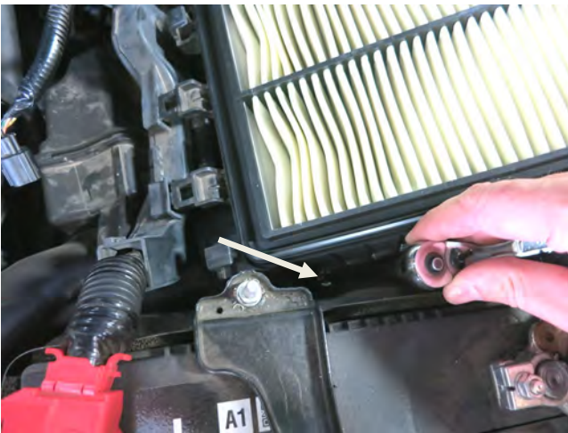
g. Use an extension and 10mm socket to reach the lower air box bolt in the location shown.
