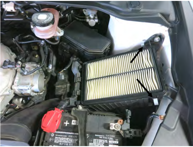
e. Unlatch the air box lid clasps and lift the air box lid and intake air hose assembly out of the engine bay.
