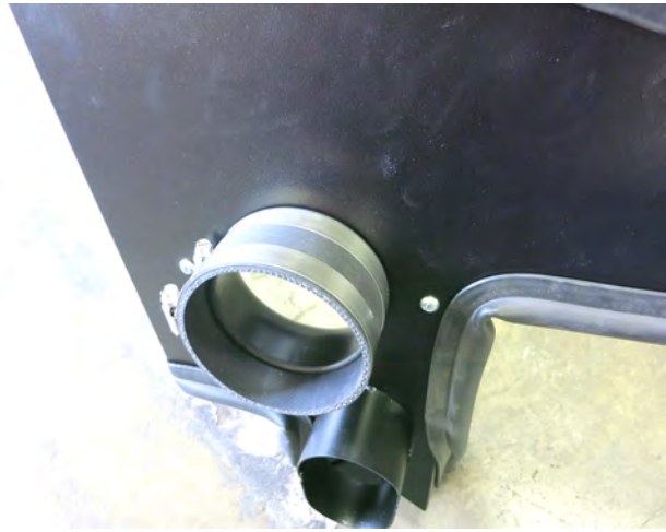
f. Attach the straight coupler to the filter adapter. Only tighten the heatshield-side hose clamp at this time.
