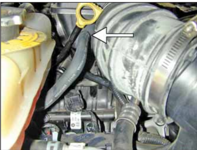
g. Detach the breather hose. Remove the remaining intake system tract.
