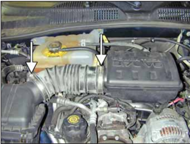
a. Loosen hose clamps.
