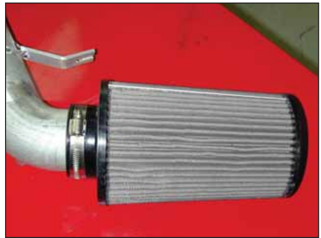
h. Attach the air filter element.
