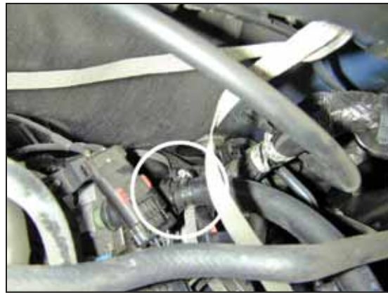
k. Attach the breather hose and secure with hose clamp.
