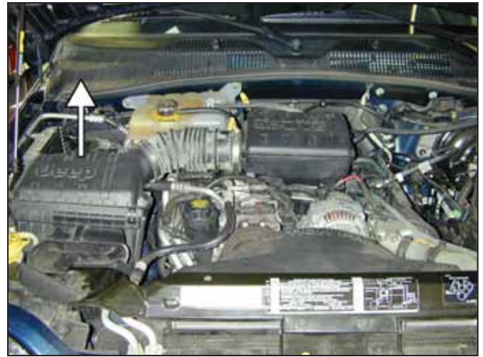
b. The air box is held in place by 3 rubber mounts on the base of the box. Gently pull out stock air box.
