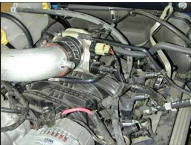
i. Insert the intake pipe and secure with the hose clamps.
