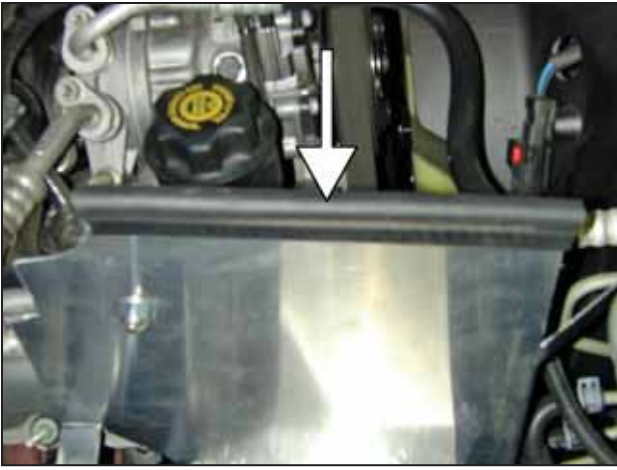
e. Attach provided rubber foam to the top of the heat shield.
