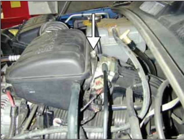
e. Loosen hose clamp.
