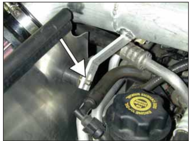
j. Secure the intake bracket to the rubber mount on the heat shield with the provided washer and lock nut. Refer to the diagram on the next page.
