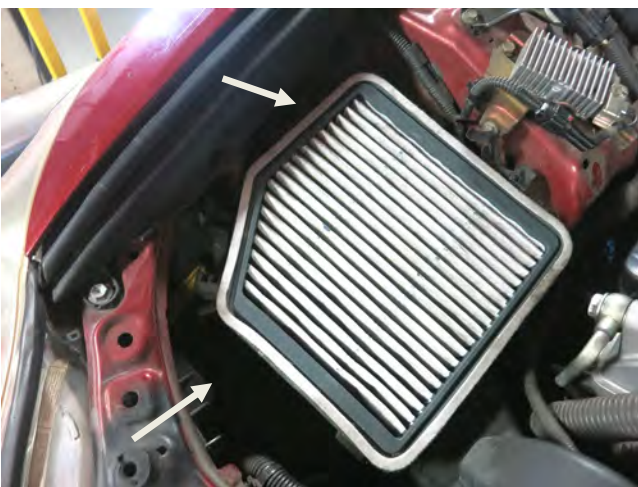
i. Remove the two bolts securing the air box base.
