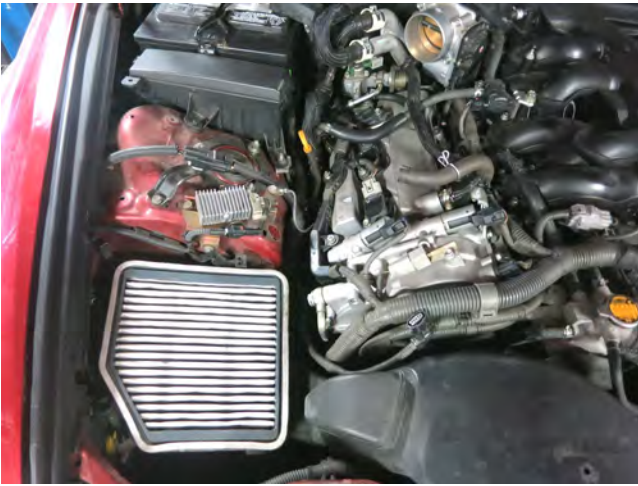
g. Unlatch the air box lid from its base and lift the air box lid and hose from the engine bay.
