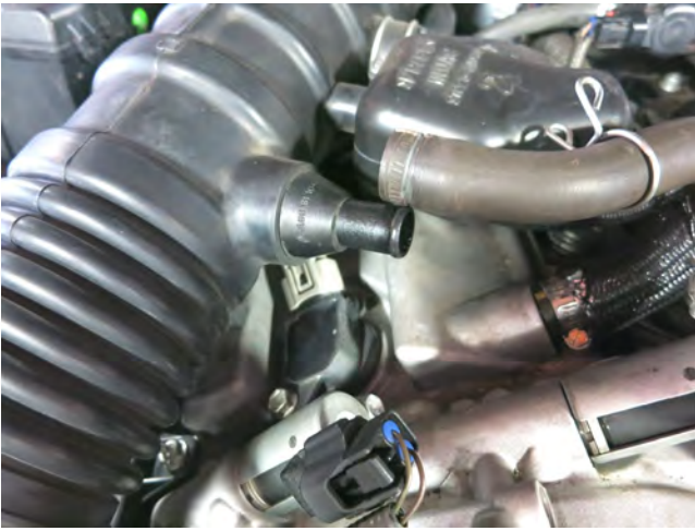
e. Disconnect the crankcase breather hose from the factory intake tract.
