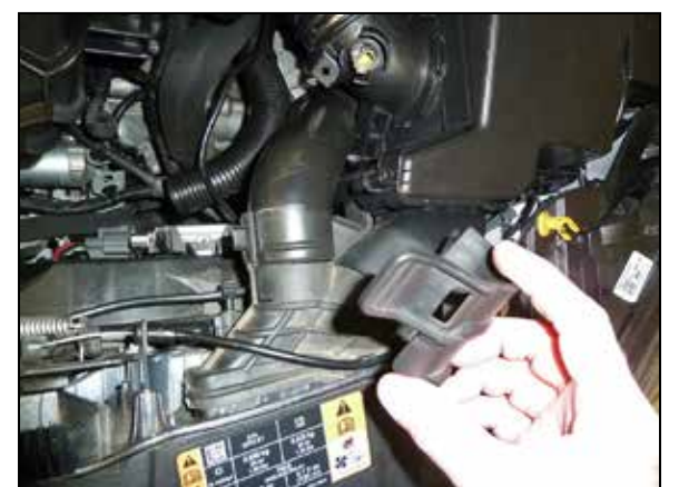
3. Unlatch the fresh air intake boot that wraps around the fresh air intake duct at the core support and remove it from the vehicle.
