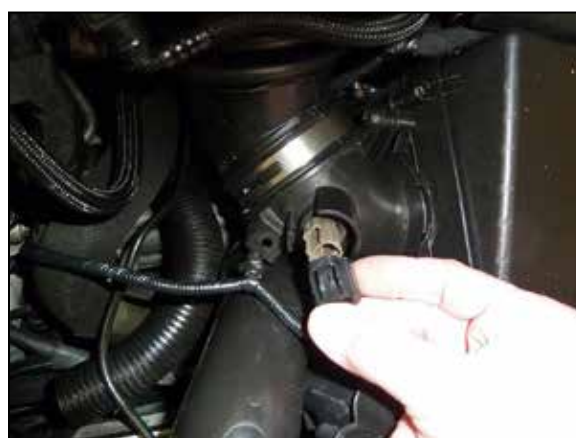
2. Disconnect the inlet air temperature sensor electrical connection.
