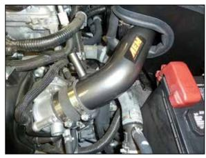
17. Install the intake tube through the heat shield and into the coupler at the throttle body. Do not tighten at this time.
