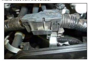
6. Release the tab on the back side of the wiring harness and then remove the harness from the bracket.
