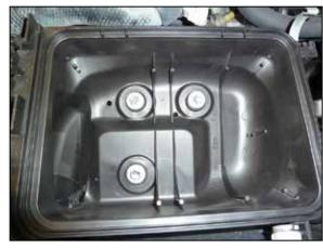
7. Remove the three bolts that secure the lower air filter housing and then remove the lower housing from the fresh air intake and vehicle.
