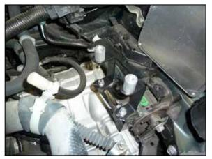
9. Install the heat shield mounting grommets as shown onto the factory air filter housing mounting location using the provided hardware.
