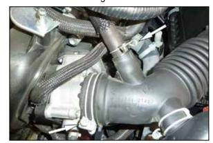
4. Release the clamp and disconnect the crank case vent hose from the intake hose. Loosen the hose clamp that secures the intake hose to the throttle body and then disconnect the hose from the throttle body.
