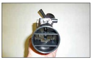
16. Using a small amount of the provided superglue on the lip of the air straightener insert, install the air straightener into the tube as shown.
