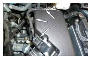
3. Disconnect the mass air sensor electrical connection and then unhook the wiring harness from the air filter housing.
