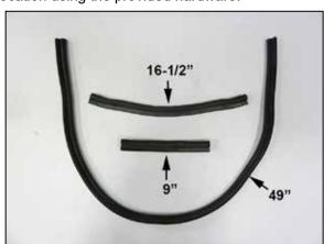
10. Cut the provided edge trim into sections of 9", 16.5" and 49" as shown.
