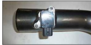
15. Remove the mass air sensor from the factory air filter housing and install it into the AEM® intake tube using the provided hardware.
