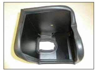
12.Install the two remaining edge trims onto the heat shield as shown.
