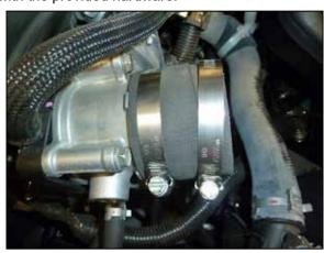
14. Install the provided coupler (5-252) onto the throttle body and secure with the provided hose clamps.
