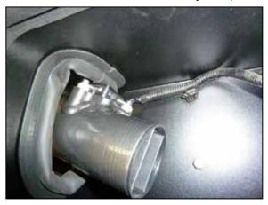
19. Connect the mass air sensor electrical connection.
