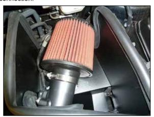
20. Install the air filter onto the intake tube and secure with the provided hose clamp. Adjust the intake tube for best fit and then secure with the provided hose clamps.
