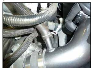
18. Connect the crank case vent to the AEM® intake tube and secure with the factory clamp.
