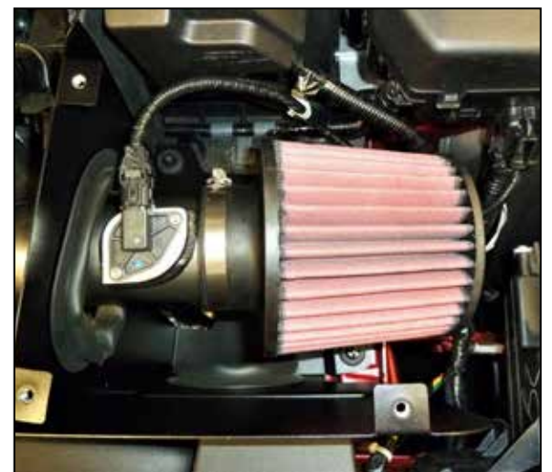
16. Install the AEM air filter onto the intake tube and secure with the provided hose clamp. Reconnect the maf sensor electrical connection.
