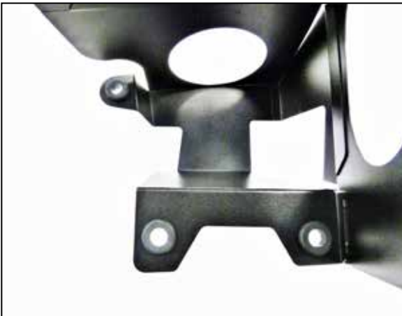
7. Install the three provided grommets into the heat shield as shown.
