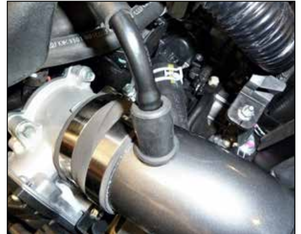
15. Install the factory ccv pipe into the grommet installed into the K&N intake tube.
