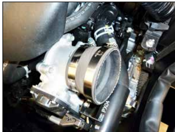
12. Install the provided coupler onto the throttle body and secure with the provided hose clamp.
