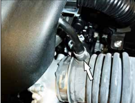
5. Loosen the hose clamp that secures the intake hose to the throttle body and then disconnect the CCV pipe from the intake hose. Lift the complete intake assembly up and remove it from the vehicle.
