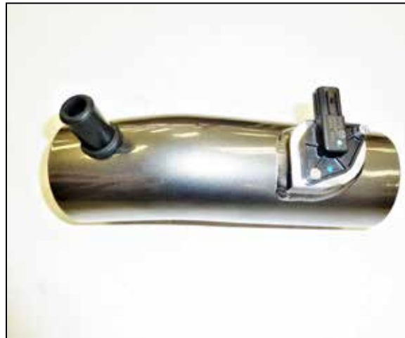
13. Remove the maf sensor from the factory air filter housing and then install it into the K&N intake tube. Install the provided ccv grommet into the intake tube and then install the provided TYPHOON decal.
