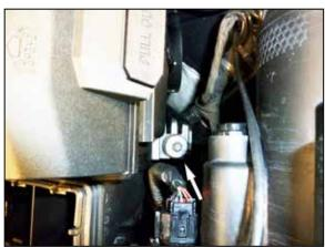
7. Remove the front air filter housing mounting bolt shown.
