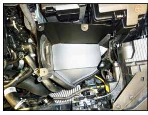
14. Install the heat shield into the vehicle and secure it to the factory air filter housing mounting location using the provided hardware.
