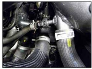
17. Connect the BOV hose and vent line to the AEM intake tube.
