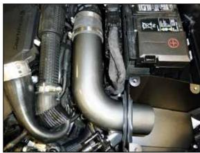
16. Install the AEM intake tube through the heat shield and then into the coupler, adjust for best fit and then secure with the provided hose clamp.
