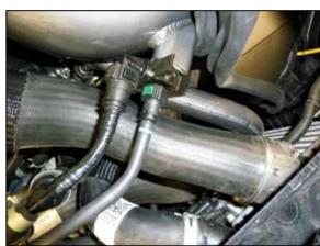
18. Connect the vent lines to the ejector fitting.
