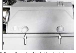
2. Pop up the center of the locking pins that secure the fresh air intake duct and then remove the pins and the fresh air duct.
