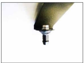
12. Install the mounting stud onto the heat shield using the provided hardware.
