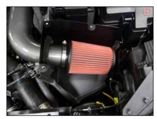
19. Install the AEM air filter onto the intake tube and secure with the provided hose clamp.
