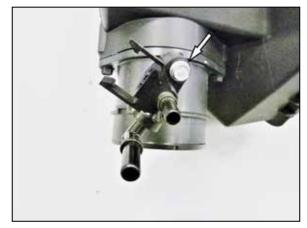
9. Remove the bolt that secures the ejector fitting to the air filter housing and then remove the fitting.
