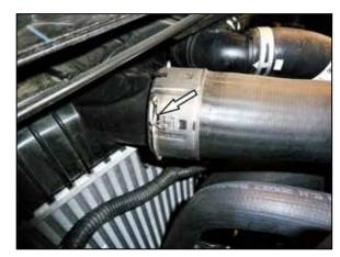
4. Spread the retaining spring securing the charge tube to the intercooler and then disconnect the tube from the cooler.
