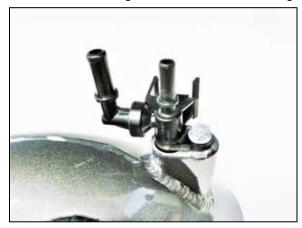
10. Install the ejector fitting onto the AEM intake tube and secure with the factory bolt.
