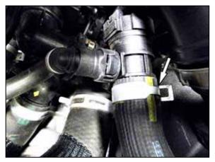
5. Release the spring clamp and then disconnect the BOV hose. Depress the locking button on the vent line and then disconnect the vent line.
