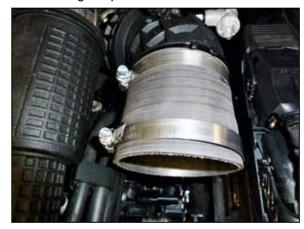
15. Install the provided coupler onto the turbo inlet pipe and secure with the provided hose clamp.
