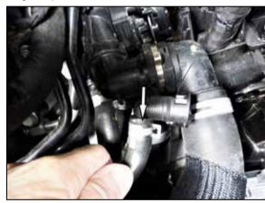
13. Release the spring clamp and remove the 90drgree quick connect fitting from step #5 and replace it with the straight quick connect fitting provided.
