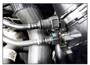
3. Depress the locking buttons on the vent lines attached to the ejector fitting and then disconnect the vent lines from the fitting.
