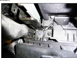
8. Remove the rear air filter housing mounting bolt shown. Remove the air filter housing from the vehicle.
