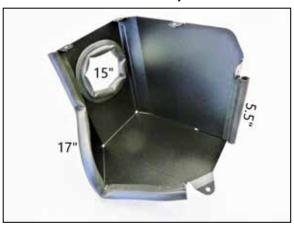
11. Cut the provided edge trim into sections of 5.5", 15", 17" and 21" long. Install the edge trim onto the heat shield as show.
