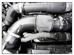
6. Loosen the hose clamps that secure the factory intake tube and then remove the intake tube from the vehicle.
