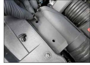
3. Pop the centers of the two push clips that secure the fresh air duct to the core support and then remove the clips from the duct.
