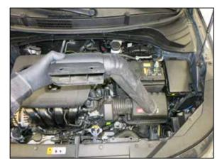
4. Lift up and disconnect the fresh air duct from the factory air filter housing and then remove it from the vehicle.
