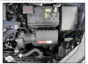
6. Remove the three bolts that secure the factory air filter housing to the vehicle.
