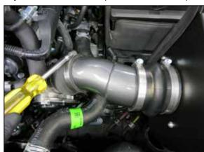
17. Install the large hump hose onto the intake tube, then install the assembly into the coupler at the throttle body, align the large hump hose with the filter adapter and slide the hose onto the adapter. Adjust the assembly for best fit and then tighten the hose clamps.
