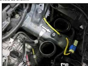
13. Install the 1" tall rubber mounted stud onto the frame rail where shown.
