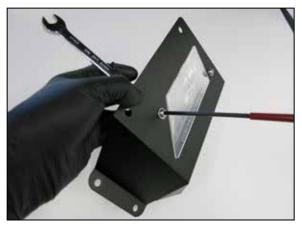
8. Install the AEM window into the into the heat shield cover using the provided aluminum spacer plate and hardware.
