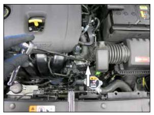
5. Loosen the hose clamp the secures the factory intake hose to the throttle body.
