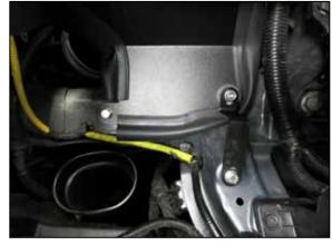
15. On 2018 and earlier models, install mounting bracket p/n 26545 onto the rubber mounted studs. On 2019 and later models install mounting bracket p/n 020003.
