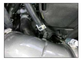
18. Connect the CCV hose to the 90-degree fitting installed into the intake tube and secure with the factory spring clamp.
