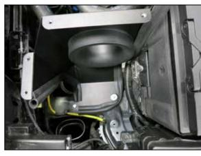
14. Install the heat shield into the vehicle and secure with the provided hardware.
