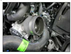
16. Install the provided coupler onto the throttle body and secure with the provided hose clamp.
