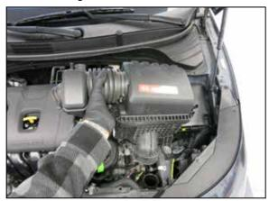
7. Separate the intake tube from the throttle body and then lift the entire factory intake system out of the vehicle.
