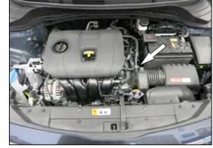
2. Release the spring clamp that secures the CCV hose to the factory intake tube and then disconnect the CCV from the intake tube.
