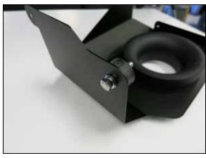
11. Install the provided  $\frac{1}{2}$ " tall rubber mounted stud onto the heat shield using the provided hardware.
