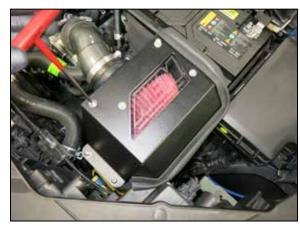
20. Install the heat shield lid onto the heat shield and secure with the provided hardware. Install the excess edge trim onto the lid as shown.
