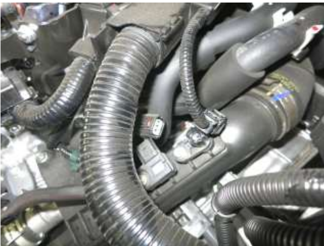
c. Disconnect the manifold absolute pressure (MAP) sensor and intake air temperature (IAT) sensor harnesses.
