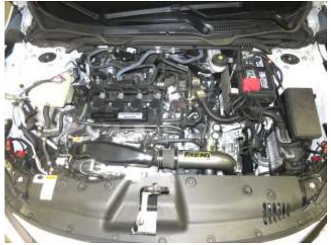
AEM CHARGE PIPE INSTALLED
