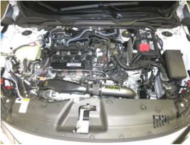
STOCK CHARGE PIPE INSTALLED
