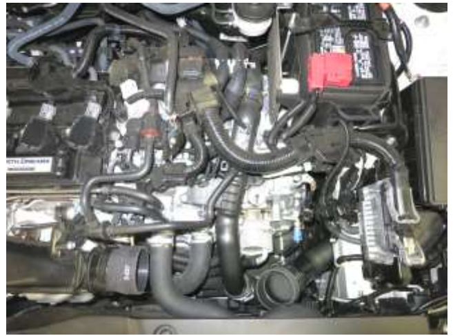
b. Loosen the hose clamps securing the upper AEM intake tube; one on the turbo inlet pipe coupler and one on the upper and lower intake tube coupler. Then, pull off the upper intake tube.
