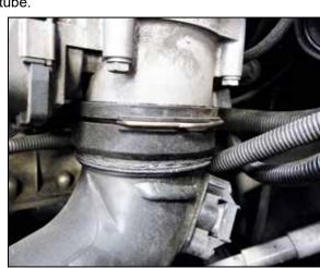
13. Remove the spring clamp that secures charge tube to the manifold inlet.
