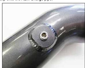
17. Install the pipe plug into the charge pipe using pipe sealant.
