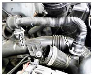
8. Rotate the grey locking ring securing the BOV tube to the intake tube counterclockwise and disconnect. Rotate the grey locking ring securing the BOV the charge tube clockwise and then remove the BOV hose from the vehicle.
