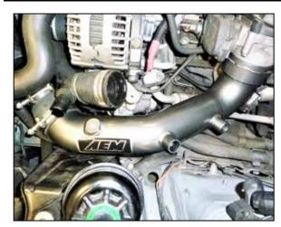
19. Install the AEM charge pipe into the coupler and then onto the manifold inlet. Be sure the locking spring secures the pipe to the manifold and then tighten the hose clamp.
