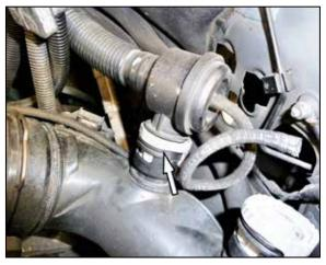
9. Rotate the lockring securing the remaining BOV valve clockwise and disconnect the valve from the charge pipe.
