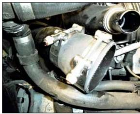
18. Install the step coupler onto the inter cooler and secure with the provided clamp.
