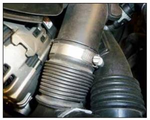
5. Loosen the front intake tube hose clamp and then pull the intake hose away from the air filter housing.
