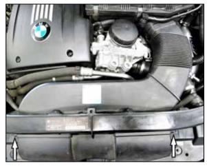
2. Remove the two screws that secure the fresh air intake duct and remove the fresh air duct.
