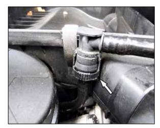
4. Squeeze the locking ring to release and then pull up the CCV hose to disconnect it from the fitting.
