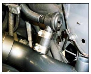
21. Using one of the provided couplers connect the BOV valve to the AEM charge pipe and secure with the provided hose clamps. Be sure the vacuum line is still connected.
