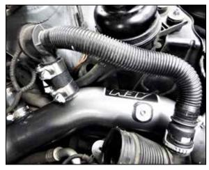
22. Using the remaining coupler and hose clamps, secure the front BOV to the charge pipe and reconnect the other end of the BOV tube.
