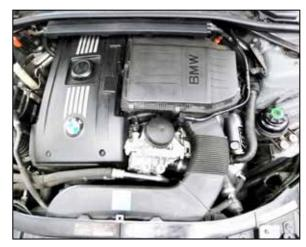
26. Reinstall the fresh air intake duct and secure with the factory hardware.
