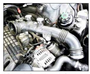
14. Remove the factory charge tube from the vehicle.
