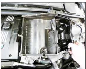
7. Pull up the lower air filter housing to disconnect it from the mounting grommets and remove it from the engine.
