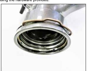
16. Remove the O-ring from inside the factory charge tube and then install the O-ring and spring clip onto the AEM Charge pipe.
