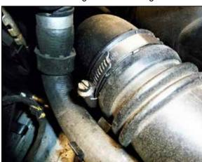
12. Loosen the hose clamp securing the charge tube.
