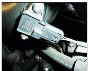
20. Reconnect the pressure sensor electrical connection.
