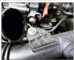
11. Remove the charge tube mounting bolt.
