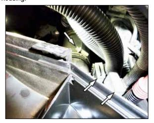
6. Unhook the three cables from the air filter housing mounting bracket, loosen the hose clamp that secures the rear intake hose and disconnect the tube.
