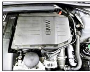
25. Reinstall the air filter and upper housing and secure with the factory clips.
