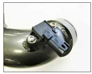
15. Remove the pressure sensor from the factory tube and then install it into the AEM charge pipe using the hardware provided.
