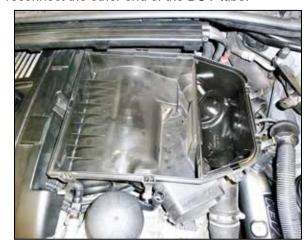
23. Reinstall the lower air filter housing onto the mounting grommets.
