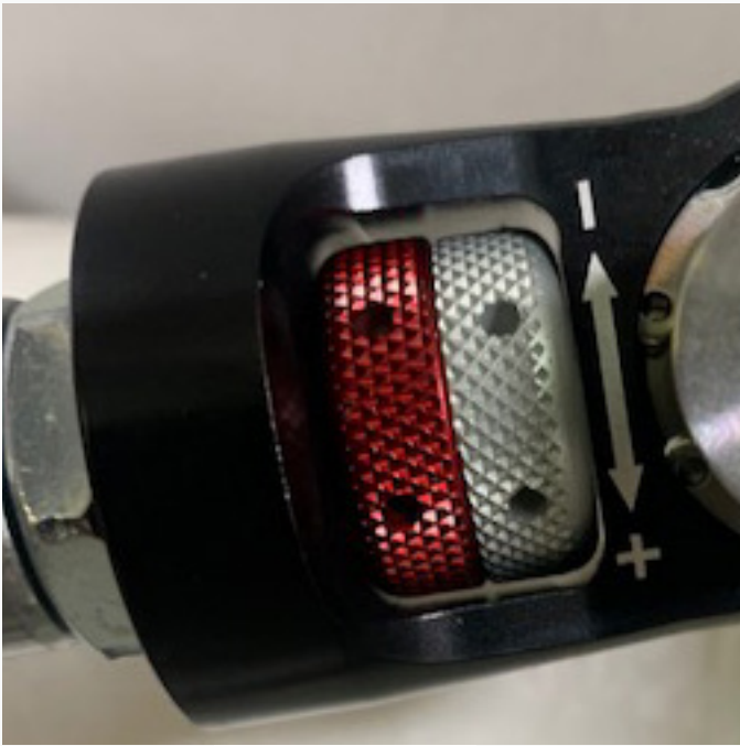
Rear Shock: Sliver Knob - Shaft Compression Red Knob - Rebound
