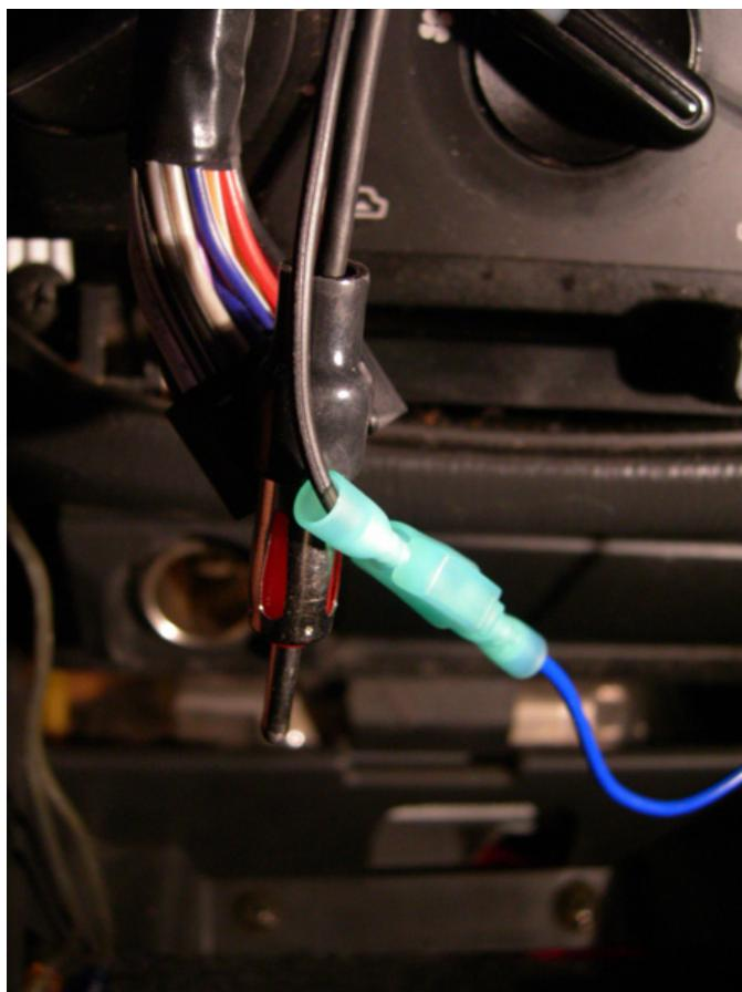
Step 10: Plug in the antenna to the back of the receiver. To test the antenna's functionality, turn the car to the on position and verify the red LED on the amplified antenna lights up when the radio is on. If it does not turn on recheck your ground and power taps. Reinstall the radio trim, kick panel, map light, and A-pillar trim. You're done. Enjoy your new stealth antenna without losing radio reception.
