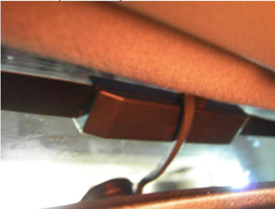
Step 6: Remove map light assembly by removing the light lens and removing the 2 Phillips screws. Pull the antenna wires through the headliner's map light hole. There will be a ground wire, a power wire, and an antenna wire.
