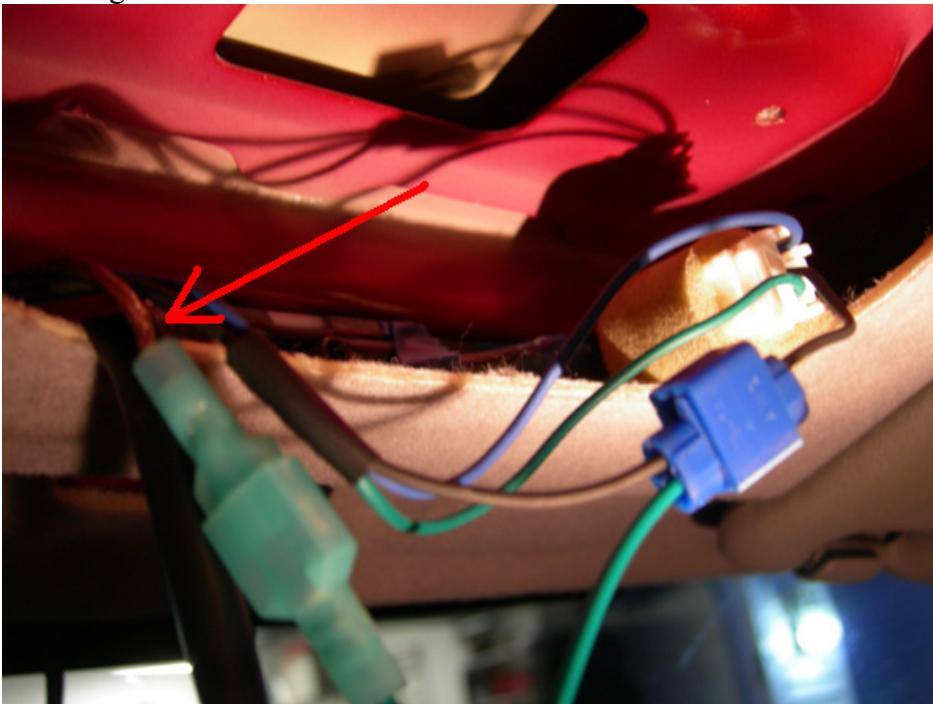
Step 8: Run the power wire and antenna wire to the "A" pillar via the headliner and down under the dash. Run it over to the radio hole where you will tap the power and plug in the antenna.
