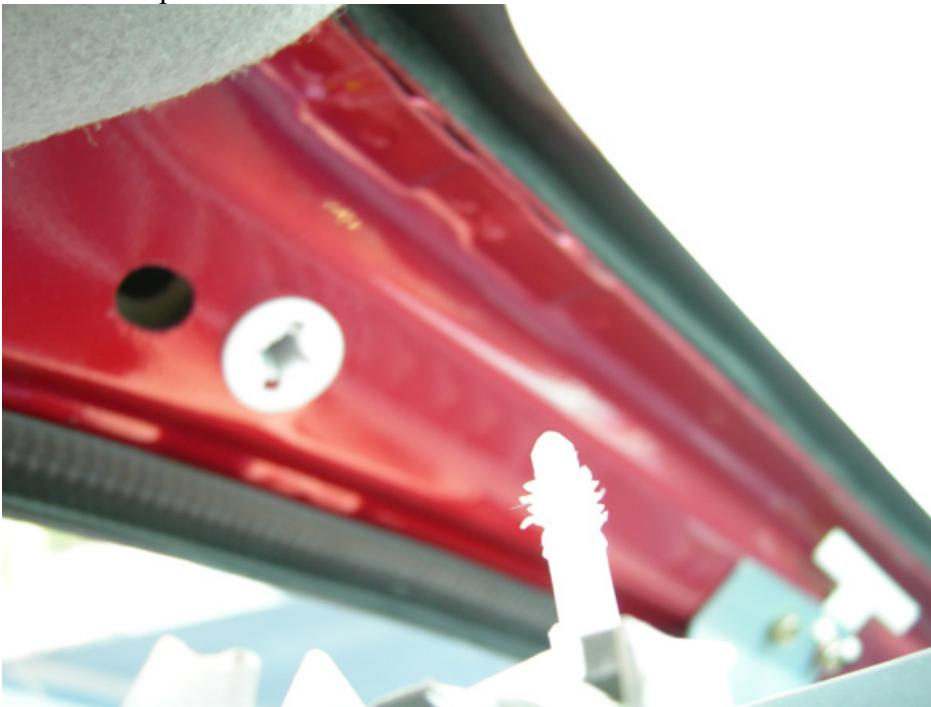
Step 3. Remove the radio and unhook the antenna from the back of the radio. Pull the cable back out the "A" pillar.
