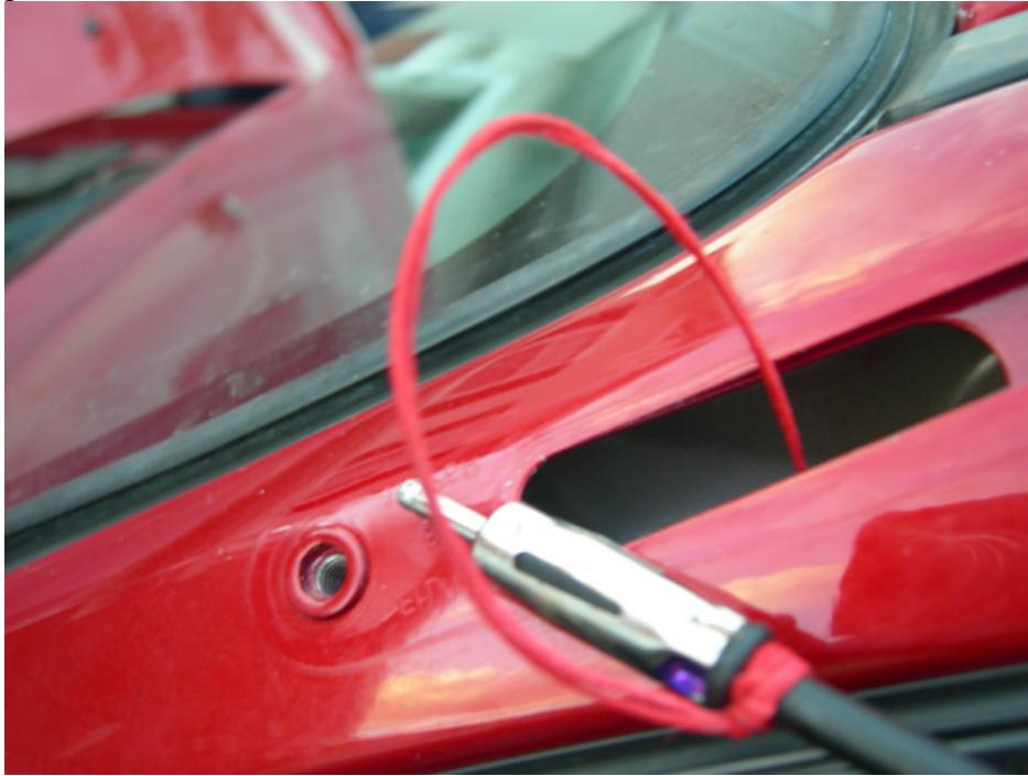
Step 4: Using the saved fasteners and gasket, install the block off plate on the A-pillar next. If you did not buy the optional antenna, reinstall A-pillar and kick panel and you're done with the plate install. If you purchased the optional amplified AM/FM antenna go to step 5.
