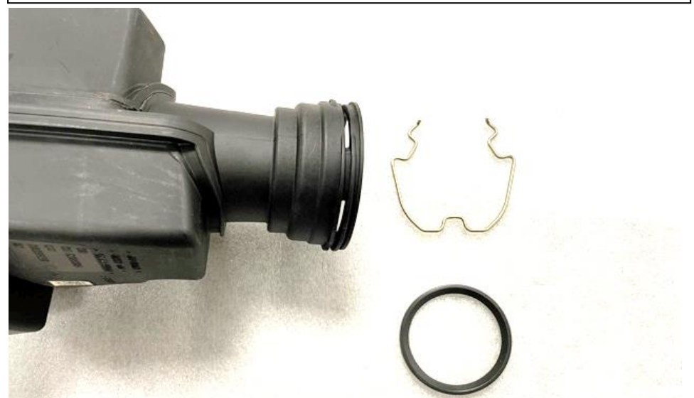
8. Remove the clip and the internal ring gasket from the OEM tube at the turbo side. Note the orientation of the gasket before removal - it needs to be in the same direction on the new flange.
