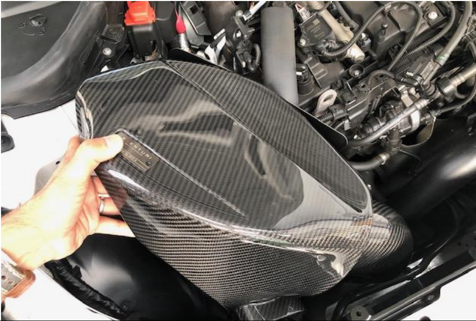
17. Carefully lower the airbox - will be easier without the engine cover in place.
