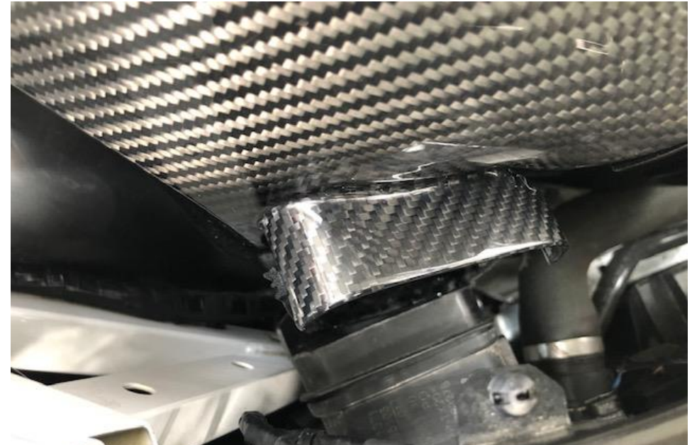
18. Bring it down at a slight angle with the front duct to locate the mounts and the secondary scoop as above.
