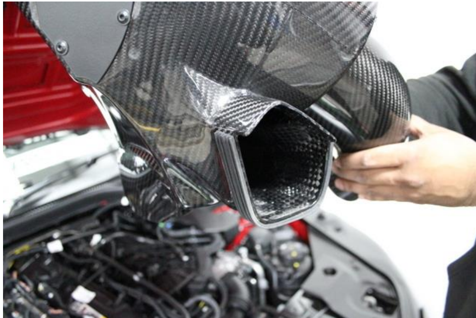
15. The main opening of the airbox should sit inside the stock duct – next photo.
