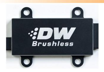
The DW Brushless Pump Controller is included with the DW440 and DW650iL fuel pump kits. This controller accepts an 8-22v DC input and creates a digital signal to allow effecient and precise speed and torque control of the pump. The controller is available in 3 configurations: C102 (Dual Speed DW440), C103 (PWM controlled), and C105 (Dual Speed 650iL)
