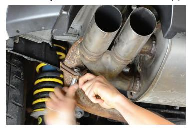
3. Next remove the two bolts connecting the downpipe to the mid-pipe.
