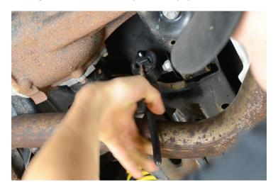
5. With the bolts and the hanger removed, the mid-pipe should be able to be pulled down and removed from the car.
