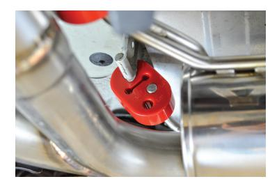
12. Now install the intermediate pipe on the OEM hanger.
