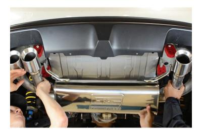
11. Push the exhaust hangers into the mounting holes as far as you can.
