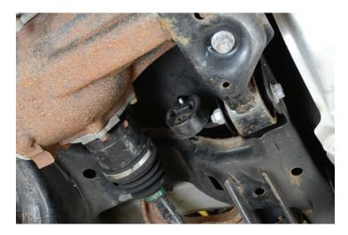
6. Now take the muffler section off the car by undoing the four exhaust hangers.
