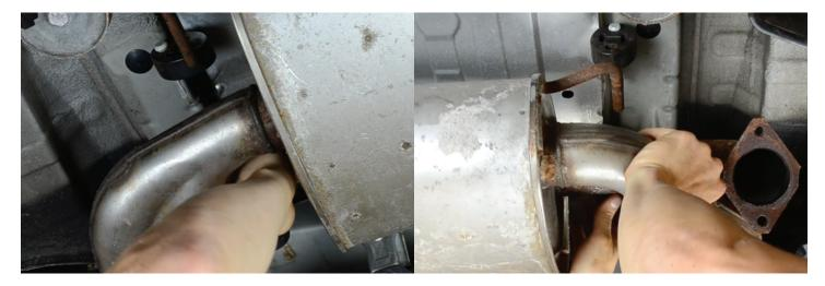
7. Our kit includes four new GrimmSpeed Poly Exhaust Hangers. You can remove the OEM hangers from the car.
