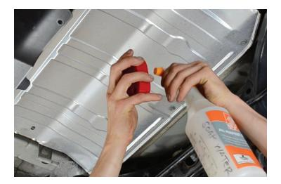
9. Once all the hangers are in place, use your soap and water mixture to lubricate the other mounting holes.
