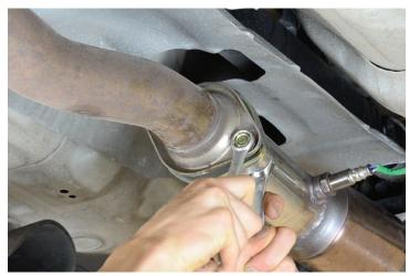
4. Now undo the exhaust hanger. You can use a pliers to pry the bracket out of the hanger.
