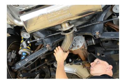
13. Using the included bolts, nuts and gaskets, bolt up the intermediate pipe to the muffler section.
