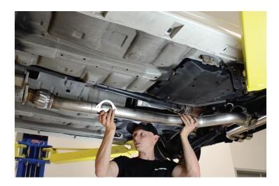
15. Using the included hardware and gaskets attached the mid-pipe to the intermediate pipe. Then bolt up the downpipe to the mid-pipe.
