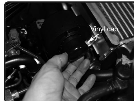
6. Install the provided vinyl cap to the sound tube accessory port.
