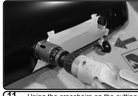
11. Using the crosshairs on the cutting template as a guide, use a 1 3/4" hole saw and drill out the two holes on the template. Make sure you drill past the second layer of the hood. Please use caution!!!
