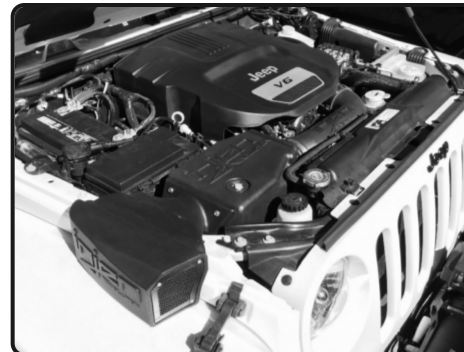
7. Injen intake system and air scoop installed.
