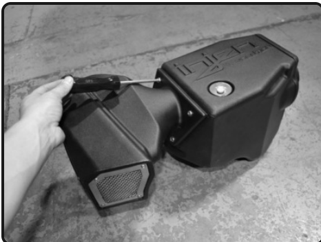
5. Place the Injen air scoop into the opening on the Injen air box and use 4-M6X20 bolts to secure the scoop to the Injen air box with a phillips screw driver.
