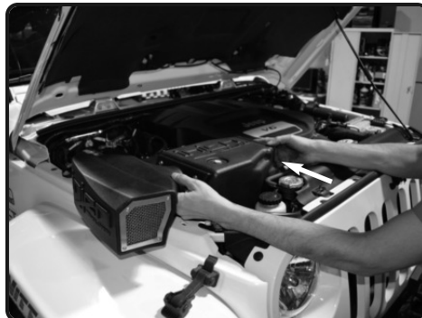
6. Once the Injen air scoop is assembled onto the Injen air box, re-installed the Injen air box and re-connect the intake tube and 4.0" hump hose from figure 2
