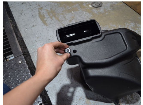
21. Install the OEM grommet on to the Injen airbox.
