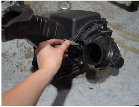
26. Twist the IAT sensor to remove the sensor from the air box.
