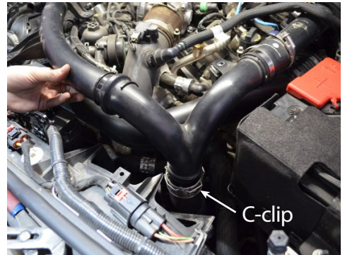
6. Pull back the charge pipe C-Clip and then lift up the charge pipe.
