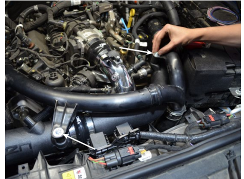
42. Secure the charge pipe to the intake tube using the provided M6 nut and washers.
