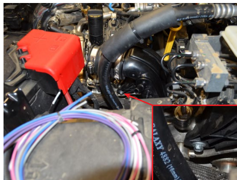
11. Remove the bolt securing the driver side intake tube to the engine.
