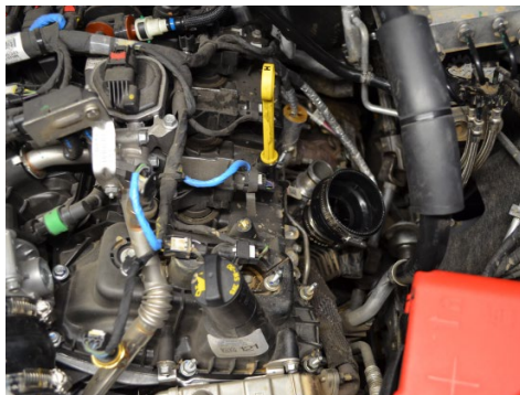
32. Attach the 2.25"-3.00" Stepping hump hose onto the driver side turbo inlet. Secure the hose with the provided clamps.
