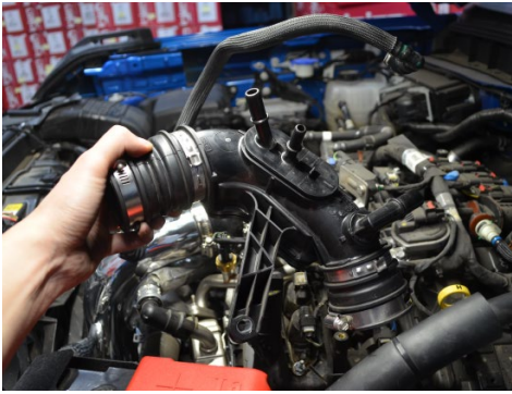
13. Loosen the clamp securing the driver side tube to the turbo inlet and then remove the tube.
