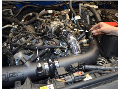
38. Install the provided M6 vibra mounts to the driver and passenger side tube.
