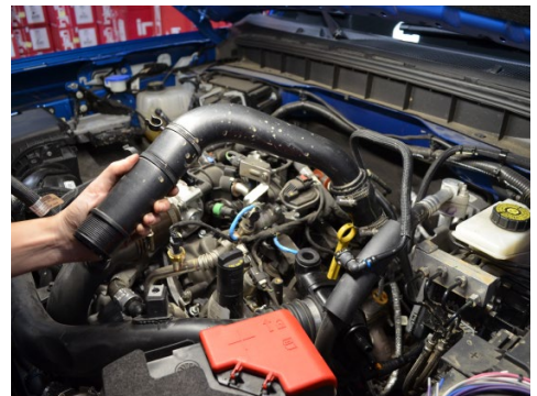
9. Remove the driver side charge pipe.
