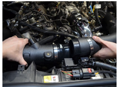
33. Attach the 3.00" hump hose to the passenger side tube then insert the driver side tube into the hump hose.
