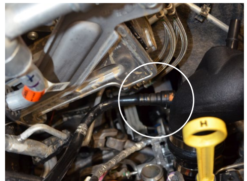
36. Reconnect the driver side crankcase line to the 5/8" machined fitting.
