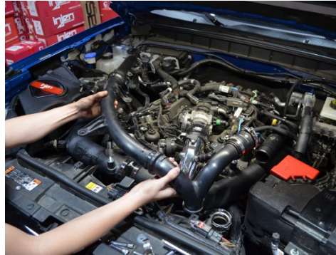
41. Reinstall the charge pipe.
