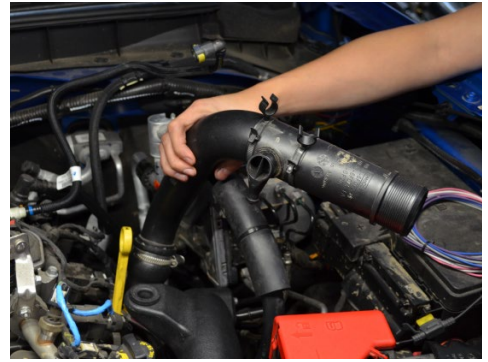
39. Reinstall the driver side charge pipe.
