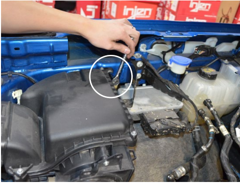
16. Remove the bolt securing the airbox to the chassis.
