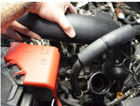
34. Insert the driver side tube into the 2.25"-3.00" Stepping hump hose.
