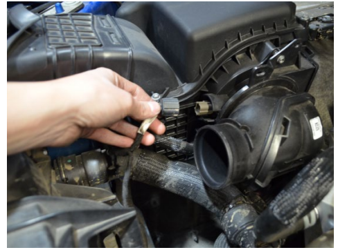
15. Disconnect the IAT sensor harness.
