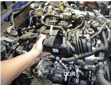
19. Remove the bolt securing the passenger side tube to the engine. Then detach the tube from the turbo.
