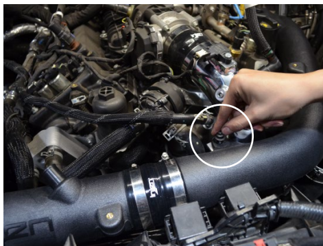
35. Secure the driver side tube to the cold side charge pipe using the factory bolt.
