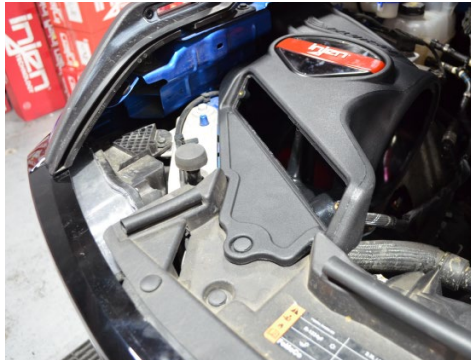
23. Secure the air box to the front shroud with the factory push clip.
