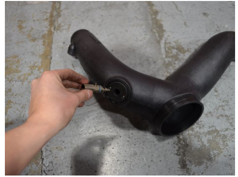
27. Install the IAT sensor to the adapter. Once fully seated, rotate the sensor to secure in place.
