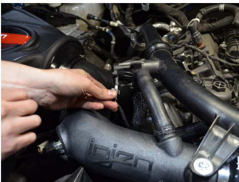
46. Reconnect the diverter valve harness.
