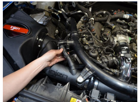
45. Connect the OEM diverter valve hose to the Injen intake and diverter valve.
