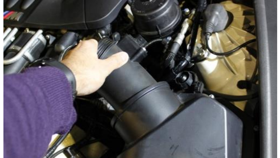
6. Pull the airbox upwards from the tube to release it from the push fit mounting points. Be careful to move any pipes out of the way. The airbox can be completely removed from the engine bay.
