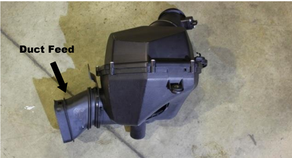
7. The complete airbox should look like this – complete with the duct feed.
