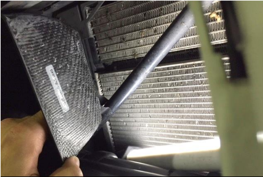
36. Place the LHS scoop inside the bumper and position the clips over the strut brace.
