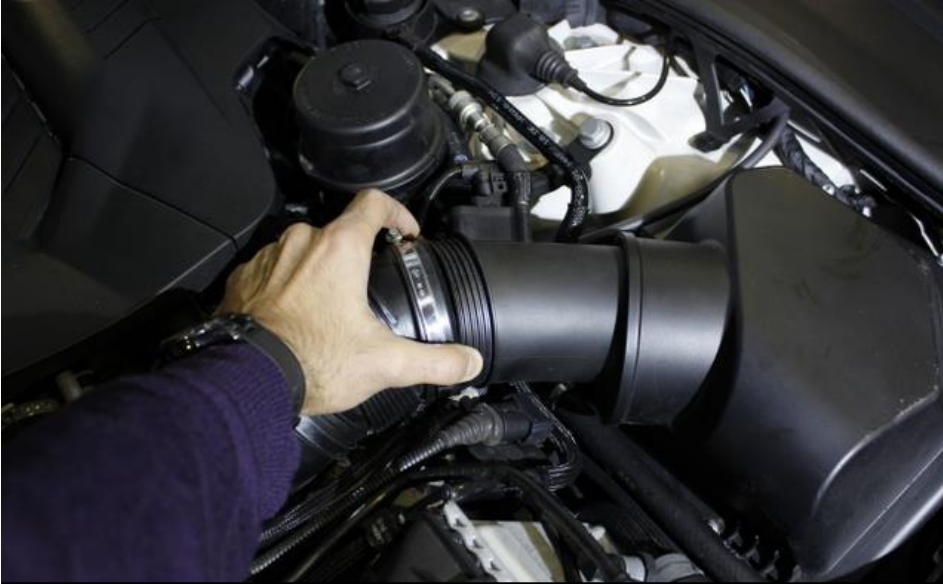
5. Loosen hose clamp around the airbox and pull the plastic inlet tube off the airbox.
