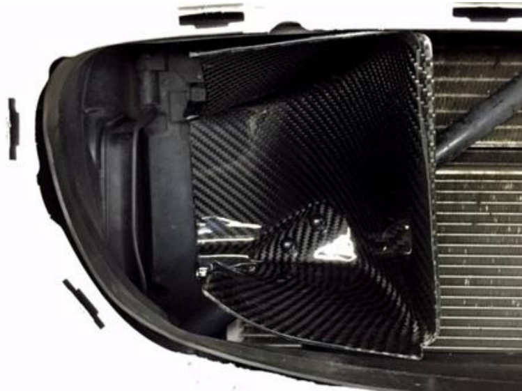
38. Now slide the scoop downwards so the lower carbon flap meets the rubber trim as shown in the next photo.
