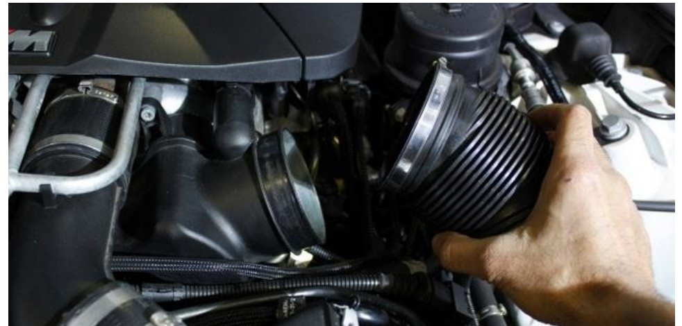
8. Now loosen the other hose clamp on the inlet tube and remove tube completely. Repeat this process for the Left Hand Side to remove the airbox and inlet tube.
