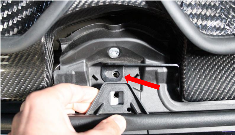
13. Pull the bumper away slightly to allow the middle bracket to sit in place.
