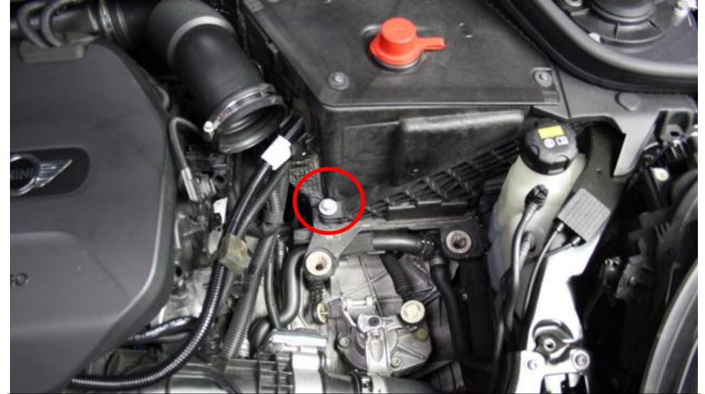
6. The airbox can now be lifted out of the engine bay. Also remove the bolt at the base of the battery tray as circled. This will be required to secure the intake later.
