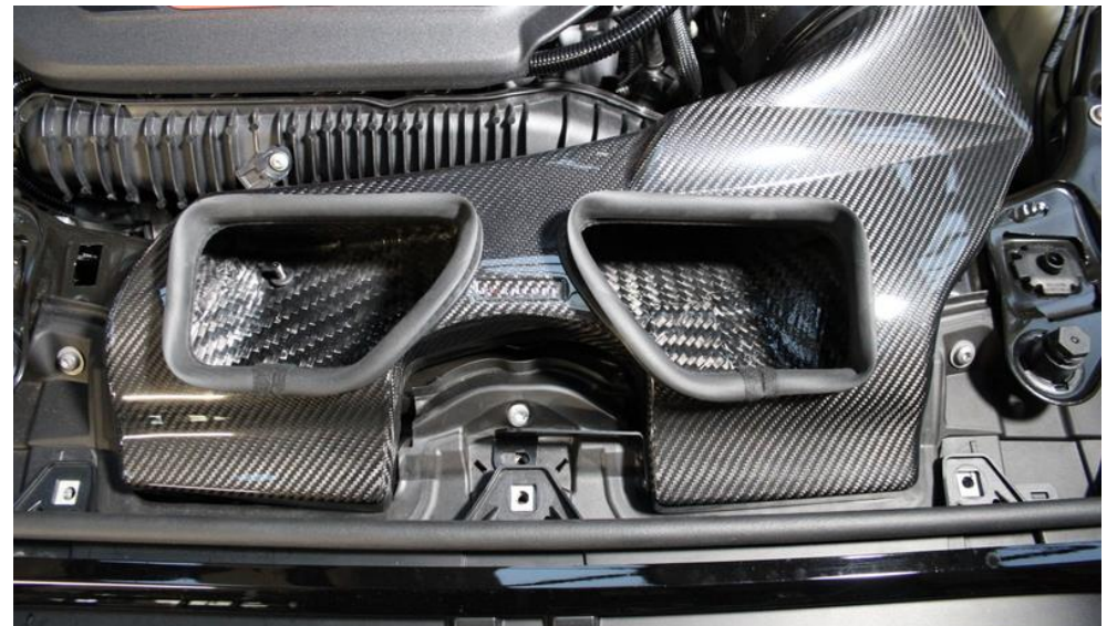
12. Push the duct into place and ensure the studs in step 8 go through the rubber grommets in step 9.
