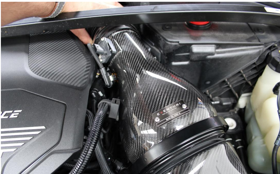
19. Line up the filter housing with the duct and then secure the bracket with the Bolt removed previously. See next step.
