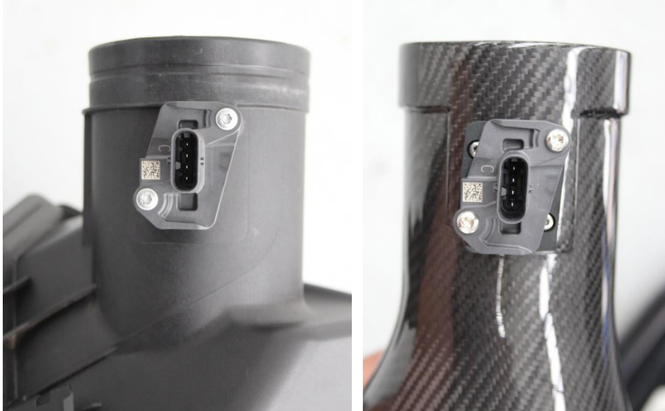
7. Remove the MAF Sensor from the stock airbox and install into the carbon housing using the supplied M4 screws. DO NOT USE THE STOCK SCREWS.
