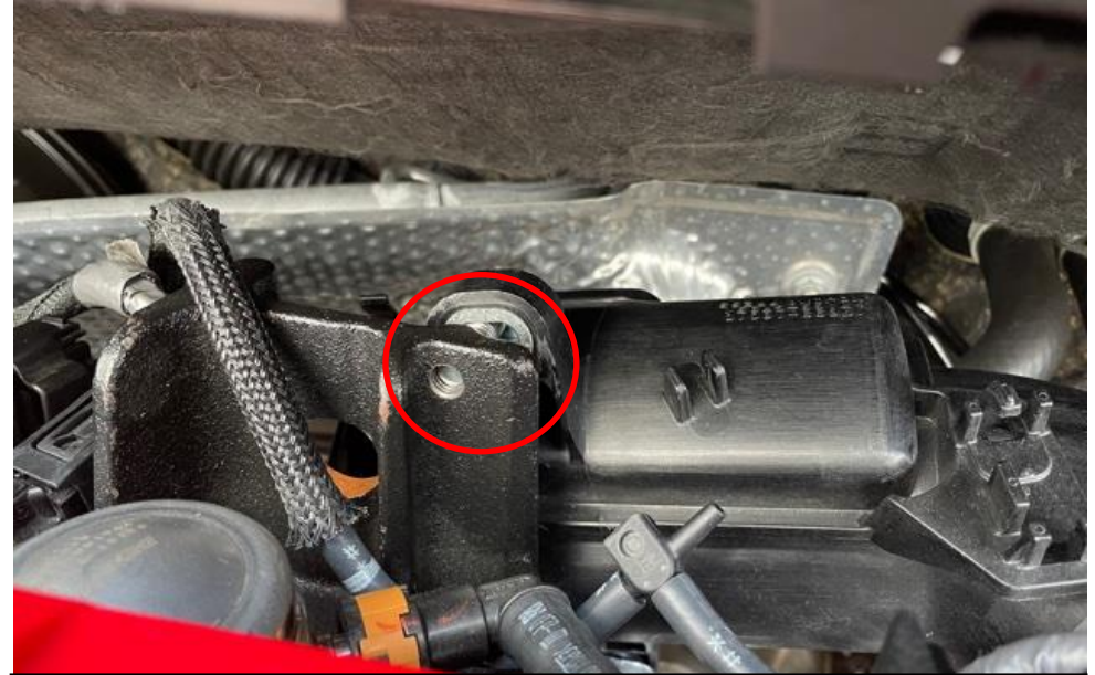
10. Move the vacuum line out of the way and remove the M8 bolt holding the top of the tube in place. There is also a second 12mm bolt on the lower side of the tube – remove this also (cannot be seen in the photo).
