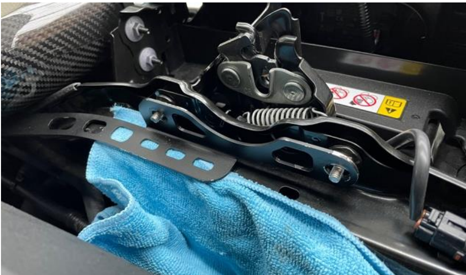
31. Position the lower bracket over the new M6 bolts installed previously. Remove the cloth.
