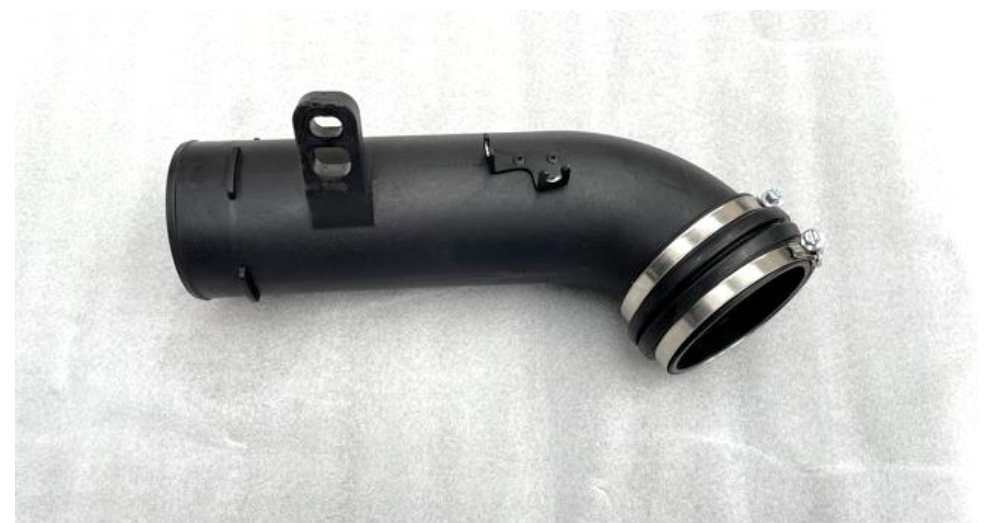
16. Push the flexible hose onto the new plastic rear tube. See next step.
