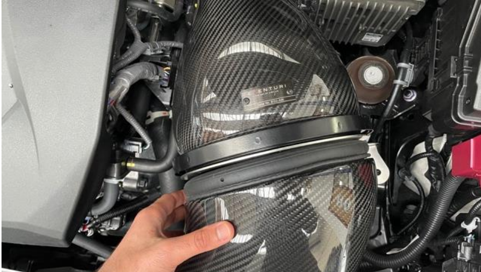
37. Line up the duct with the housing and now tighten the screw which went into the plastic clip. See next step.
