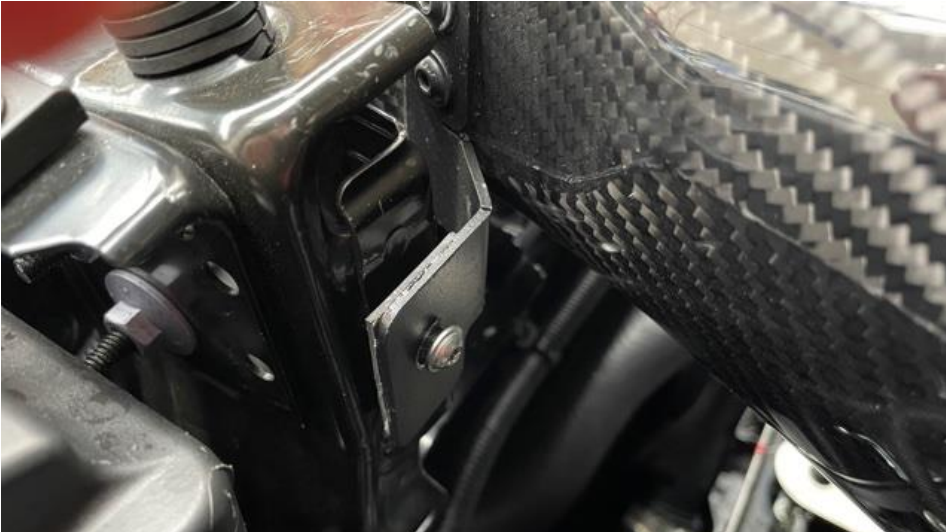
33. Screw into the white clip through the bracket but DO NOT tighten yet.
