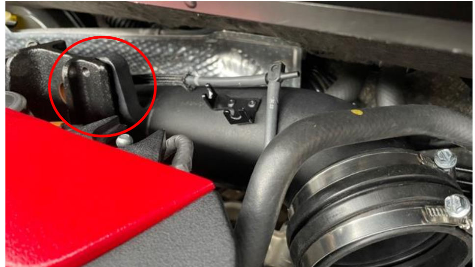
18. Insert the tube into the OEM rear rubber hose. Rotate the tube so that the tube mount lines up with the metal bracket. Do not insert the 13mm bolt yet.
