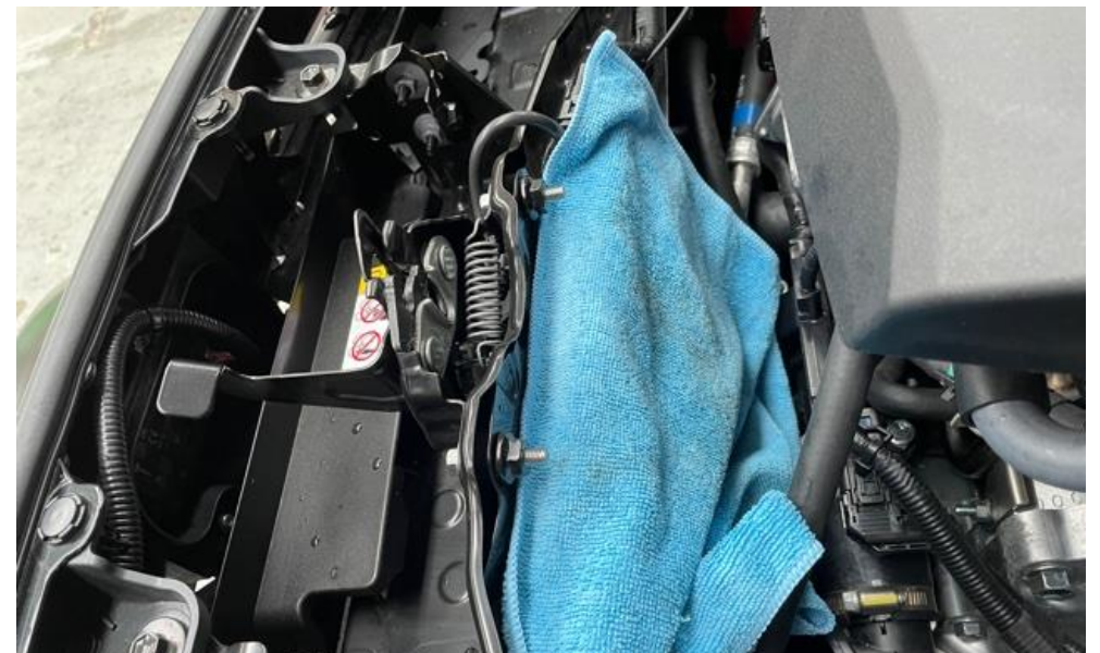
24. Place a cloth on the slam panel area for protection while installing the duct.
