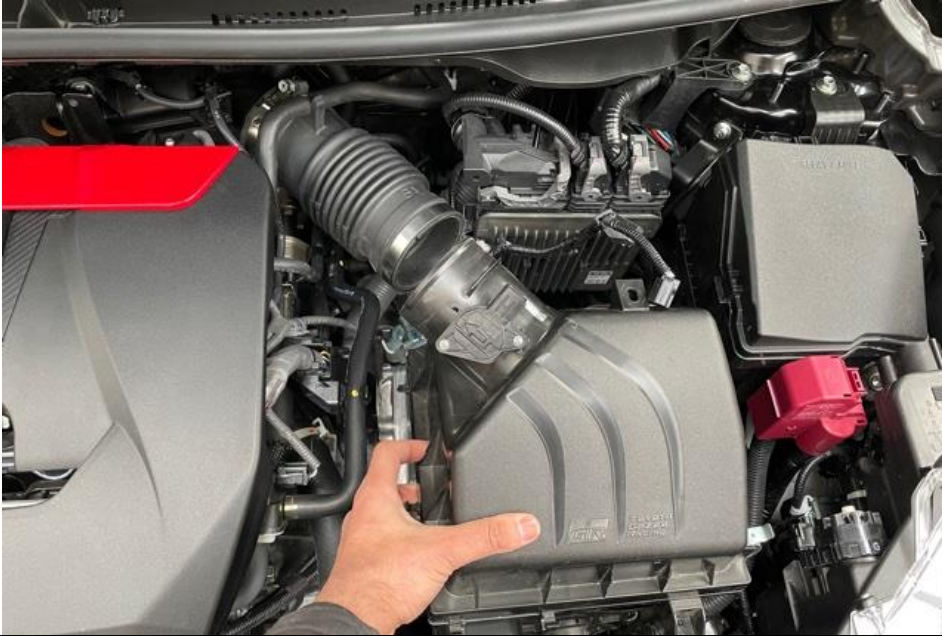
9. Loosen the hose clamp at the back of the airbox and remove the airbox from the engine bay – it can be pulled out.
