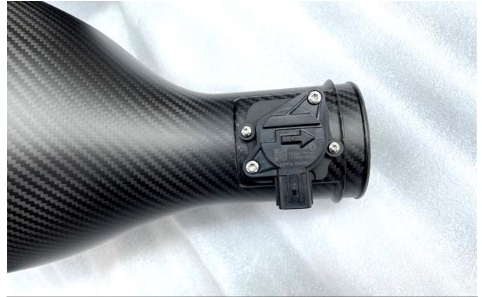
14. Install the MAF sensor to the carbon housing as shown – use the SUPPLIED M4 screws. DO NOT use the stock screws.
