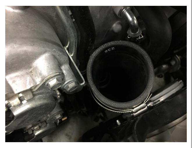
22. Take the GrimmSpeed Charge pipe, and with the logo facing up, slip one end all the way into the reducing coupler on the intercooler.
