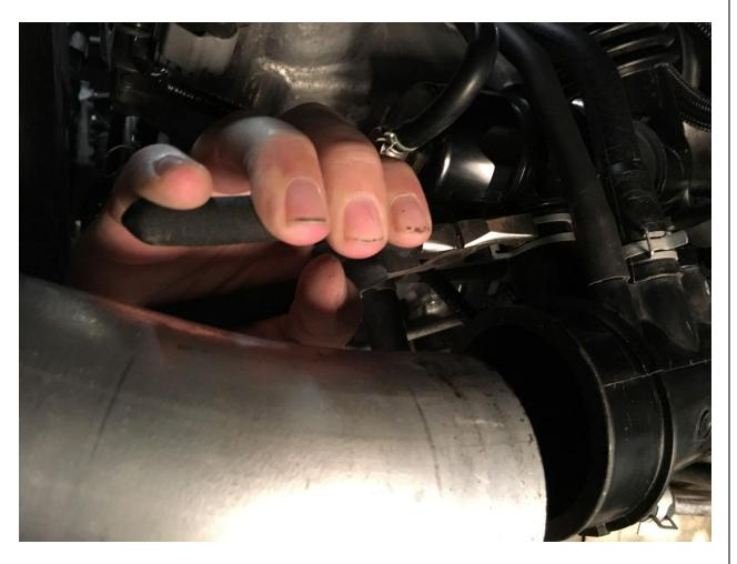
6. Loosen the hose clamp attaching the other end of bypass valve to the charge pipe with your flathead screwdriver, and move it out of the way.
