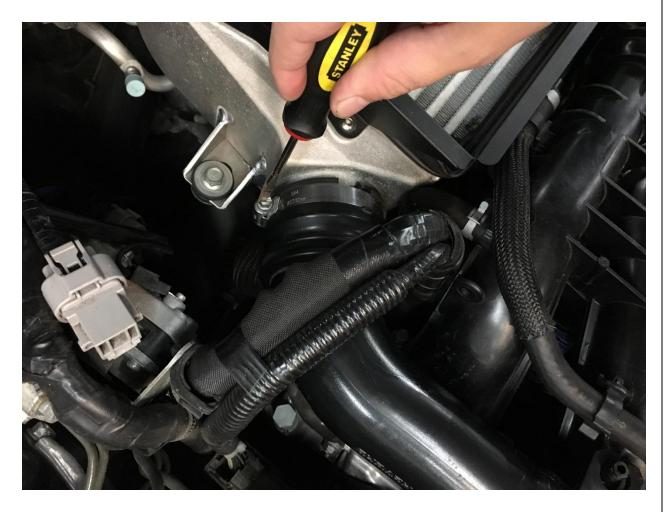
4. Now safely raise the front of the vehicle and support it with jackstands or ramps as the next portion of the installation occurs under the front of the vehicle. From there, loosen and remove the coupler attaching the intake to the turbo inlet. If your intake is OEM it will be an "accordion style" s-tube, but is removed just the same.
