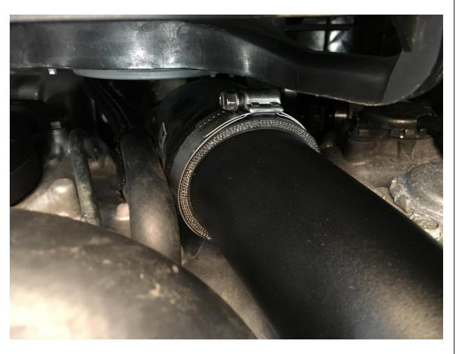
25. Check to make sure that all hose clamps are on the opposite side of the bead roll on the pipe, and that they are tight. You will be able to feel the bead roll of the pipe through the silicone with your fingers.
