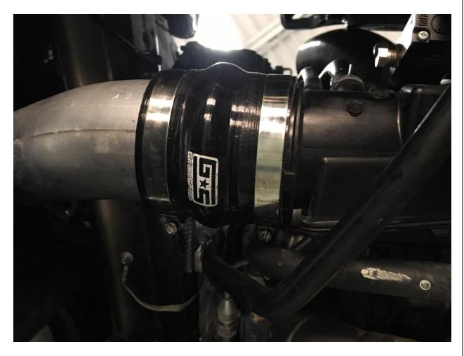
20. Locate the supplied reducing coupler as well as the largest hose clamp, and one of the two medium sized hose clamps. Place the large end of the reducing coupler onto the intercooler and place both hose clamps onto the coupler, starting with the large one. Tighten the large clamp over the coupler onto the intercooler, but leave the medium sized coupler loose.
