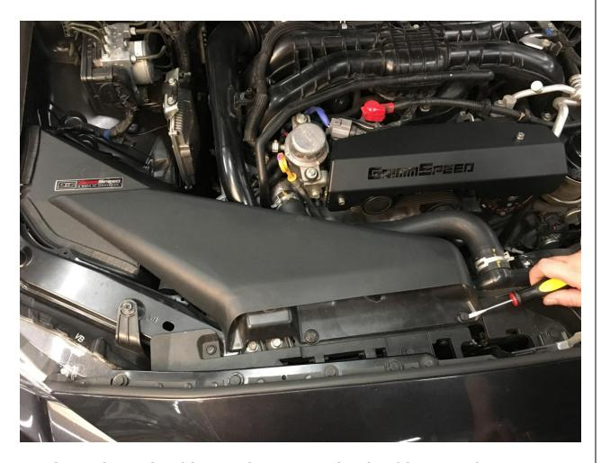
3. Next, loosen the coupler of the OEM charge pipe to the inlet of the intercooler.
