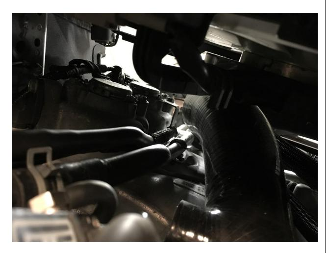
15. Verify that the silicone outlet hose is pushed all the way down on the turbo outlet adapter, and make sure that the hose clamp is in between the two 13mm bolt heads and all the way at the bottom of the silicone outlet hose, as shown in this picture. Then tighten the hose clamp.
