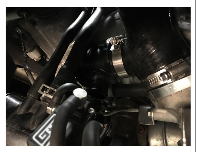
17. Grab the plastic turbo inlet, and insert the hose you removed from the bypass valve in Step 5 back onto the bypass valve all the way in. Using your pliers, replace the clamp that was removed in Step 5, and replace the small vacuum line to the "head" of the bypass valve. Using the two OEM 10mm bolts, re-attach the turbo inlet to the compressor housing.
