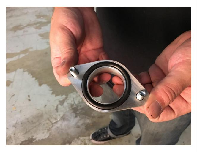
12. Place the adapter onto the compressor outlet where you removed the OEM chargepipe from the turbo. Using the supplied 13mm bolts and a 13mm socket, tighten the bolts to 11.8ftlbs.
