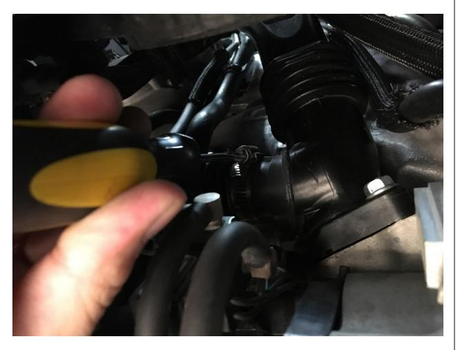
7. Remove the two 10mm bolts attaching the plastic turbo inlet to the compressor housing of the turbo.
