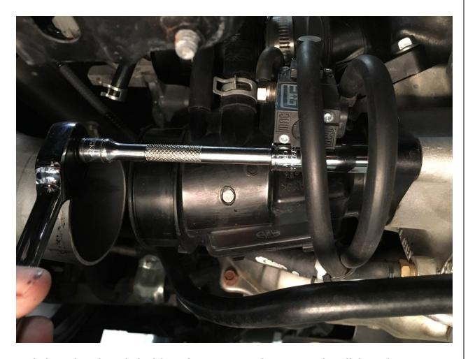
8. With the turbo inlet unbolted from the compressor housing gently pull the turbo inlet down, removing it from the bypass valve. Remove the small vacuum line going to the "head" of the bypass valve, and then remove the bypass valve itself from the charge pipe and set it aside.
