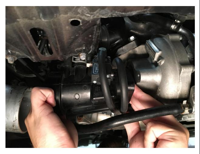
9. Next, remove the two 12mm bolts connecting the OEM charge pipe to the compressor housing.
