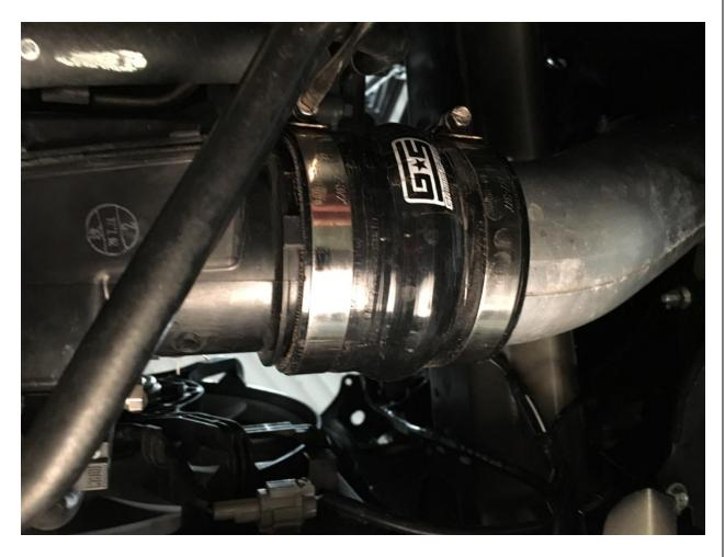
5. Using your pliers, loosen the clamp holding the bypass valve to the plastic turbo inlet, and move it down and out of the way of the bypass valve.
