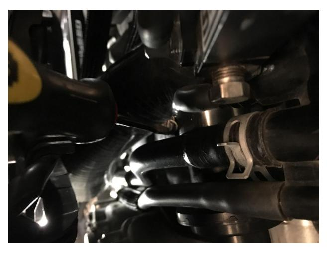
19. Re-attach your intake coupler to the turbo inlet, and tighten the clamps. You may now lower the front of the vehicle back onto the ground.
