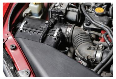
2. Find the two pop clips holding the air snorkel in place. Pop the clips and remove them, then pull the snorkel up and out. Place it aside.
