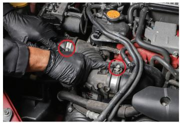
4. You may find that your OEM MAF hose is difficult to pull off. In this case you can use a flathead screwdriver to gently pry off the hose.
