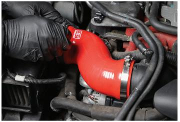
6. Reassemble the intake system by bolting the airbox back to the chassis and re-installing the snorkel.
