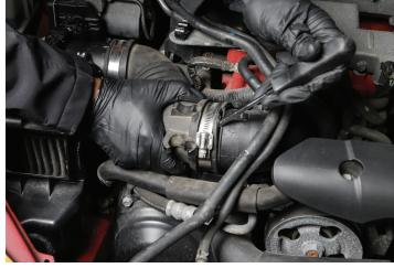
5. With the OEM hose removed, place the included worm clamps on your new GrimmSpeed Post MAF Hose and install as shown below. Make sure the hose is properly seated and the clamps are installed and tightly secured in place.
