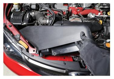
3. In order to have enough play to remove the OEM post MAF hose you will need to loosen and remove the 10mm bolt holding the intake box to the chassis. Once this is done, you can loosen the two clamps on the OEM MAF hose.
