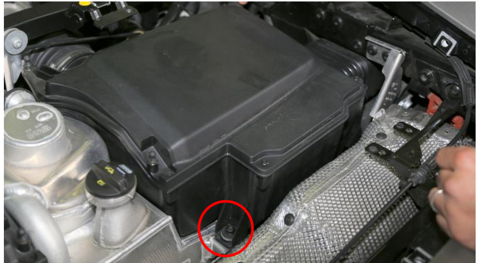
8. Remove the 4 screws holding each airbox in place. There is one screw on each corner.
