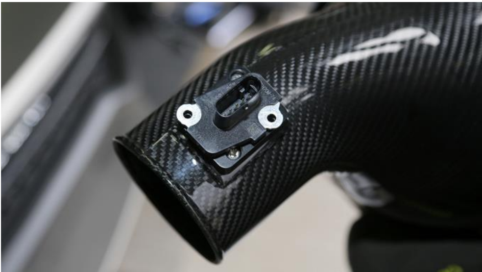
15. Insert the sensors into the Eventuri intake tubes. Make sure the orientation is correct. See next step for using the supplied spacers under the sensors.
