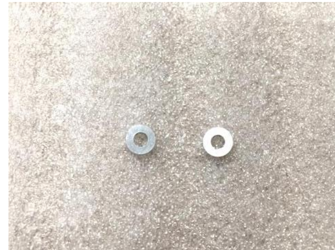
16. Take the 2 supplied M4 spacers and place them between the MAF sensor and the mount, under the securing holes.
