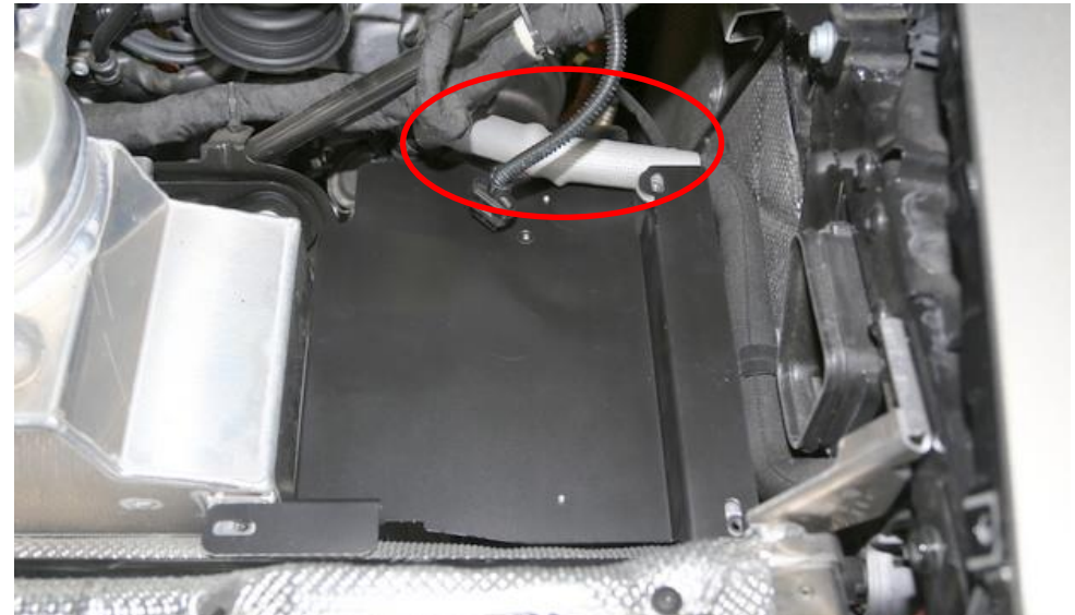
20. Take the other shield and position into the right side of the engine bay. The hose near the engine circled in red should go over the top of the shield as shown. Secure this shield using 3 screws previously removed from the airbox.
