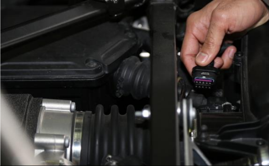
9. Disconnect the MAF sensor plugs from both airboxes.
