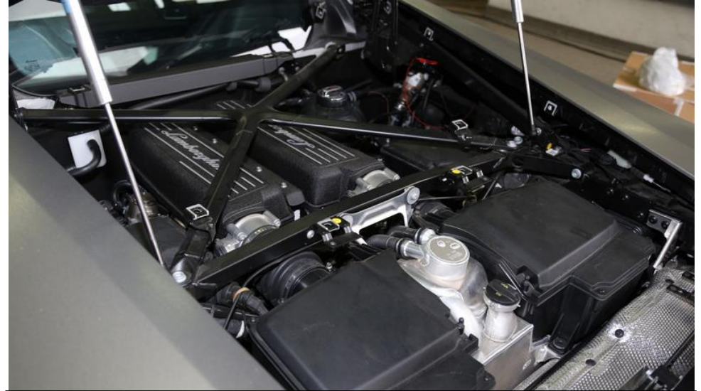
6. Remove the side covers from the engine bay.
