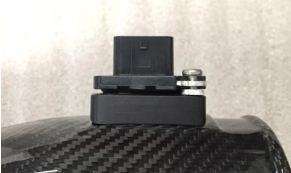
17. With the spacer in place as shown – secure the sensor with the supplied M4 screws.
