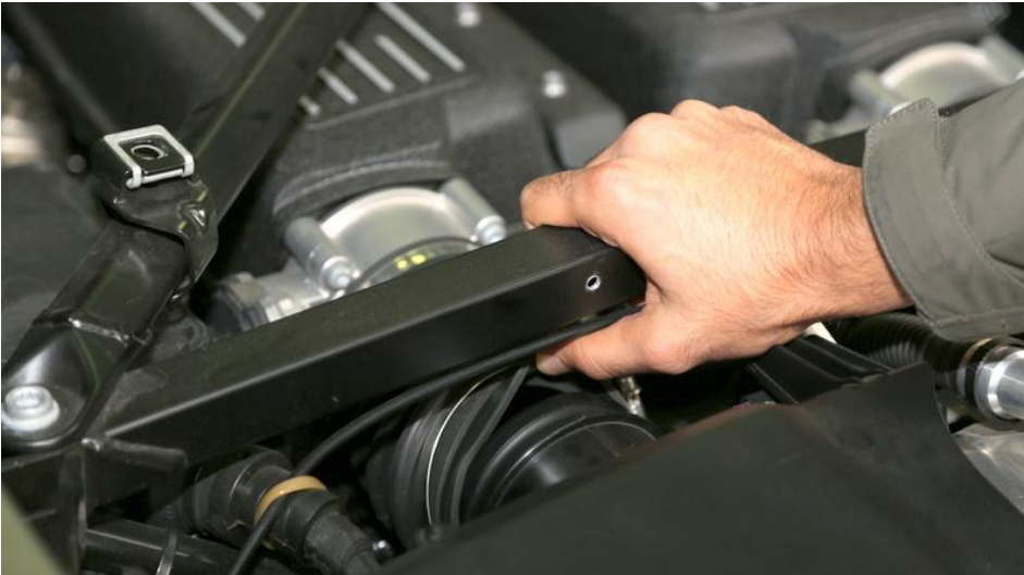
11. Loosen the hose clamp around the inlet tubes and push them off both airboxes.
