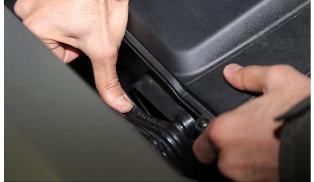
10. Push the plastic inlet duct connectors off the airboxes. They are located on the side of the airboxes nearest the wing.
