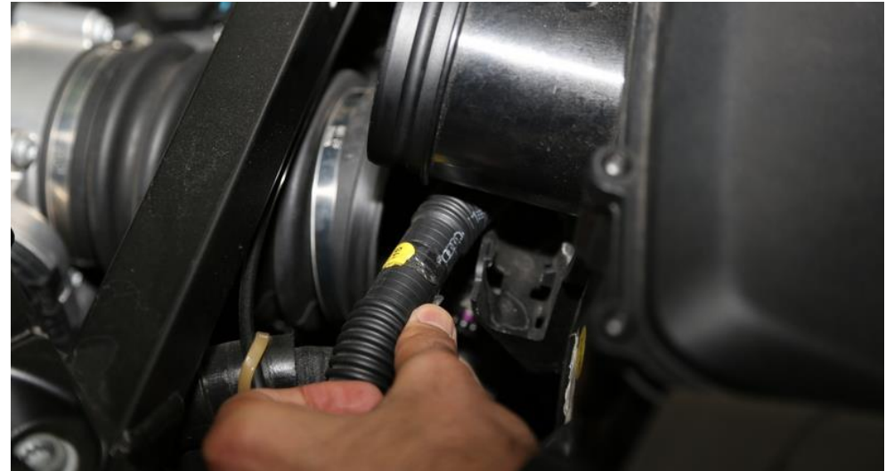
12. Now the airboxes can be pulled out. On the left airbox (as you look at the engine) there is a hose which needs to be removed from the airbox as shown. Remove both airboxes completely.
