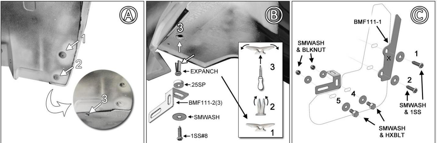
**REAR FLAP** Do not fully tighten fasteners until flap is completely aligned to vehicle.
