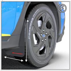
**REAR FLAP** Do not fully tighten fasteners until mud flap is completely aligned to vehicle.
