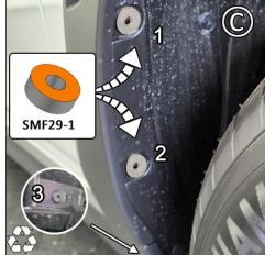
**FIGURE D/E** Place BMF106-FRT on logo-side of flap. Adhere BMF106-ST-L/R to BMF106-FRT side facing rear bumper. Install SMWASH & 1.5SS through mounts 1 & 2 and SMWASH & HXBLT through flap/bracket mount 4. Secure with BLKNUT. **FIGURE F** To enhance clearance between tire and flap, bend bottom section of BMF106-FRT towards rear bumper. Align flaps to even ground before tightening fasteners until washers just seat against flap.
