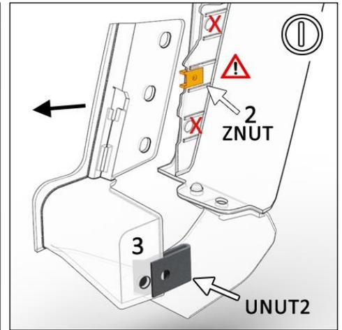
**IMAGE J** Reinstall liner and factory fastener 1.
