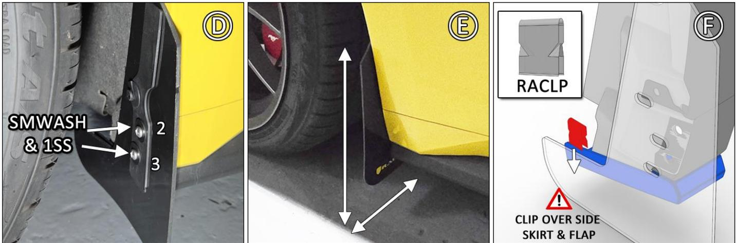
**REAR FLAP** Parts x 1 Flap → 1 x BMF126-2; 1 x .75SP; 1 x 1.5SP; 1 x 1SS; 1 x 3.5SS; 2 x BLKNUT; 2 x HXBLT;
