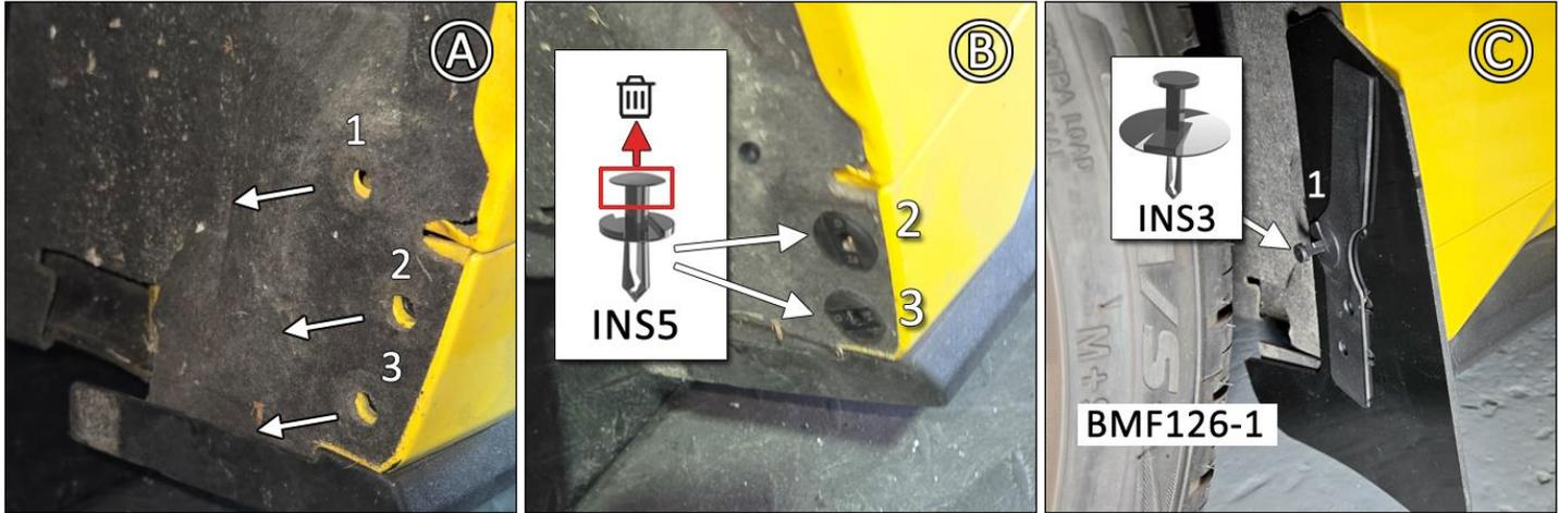
**IMAGE D** Install SMWASH & 1SS into mounts 2 & 3.
