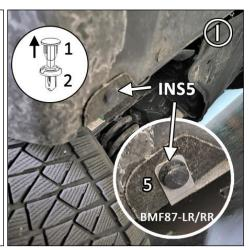
**FIGURE J** Adhere SMF29-1 to .25SP, and place **between liner & flap mount 1**. Position logo-side of flap facing rear bumper. Install SMWASH & 1.5SS into mount 1.
