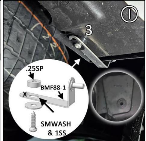
**IMAGE J** Remove film from SMF29-1 & SMF148-1/2. Attach SMF29-1 over INS10 mounts 1 & 2 and SMF148-1/2 on liner, behind stud.
