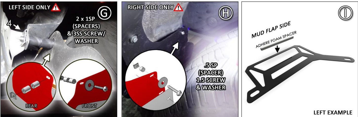
FIGURE J << LEFT REAR MUD FLAP Excluding mount #8, follow mounting process as shown in Figure J. Use a Short Screw 1SS and Washer for #8. FIGURE K >> RIGHT REAR MUD FLAP Note the right flap shares a single point with its right-side Fender Liner. Position the flap logo-side against the corresponding mounting points of the bumper. Line the Bracket up to mounts #6 & 8. Mounts #5, 6 and 8 utilize factory screws and supplied Washers. FIGURE L Make slight angle adjustments. Walk away from the vehicle to check the flap is even with the ground. Tighten mounting screws until seated against the flap.
