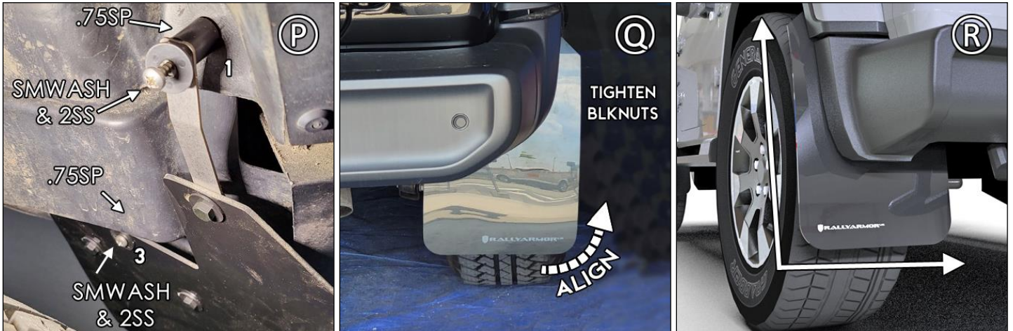
FIGURE Q/R Ensure flap is parallel to even ground. Loosen HXBLT mounts to align if necessary. Tighten washers until flush against flap.
