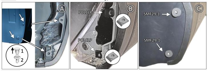
**FIGURE D/E** Place logo-side of mud flap facing rear of the vehicle against mounting points on liner. Position BMF78-FRT bracket OVER mud flap. Use WASHER SMWASH & SCREW 1SS to fasten points 1 & 2. Use a SMWASH & HXBLT and BLKNUT & SMWASH BEHIND mud flap for lower mounting point #3.
