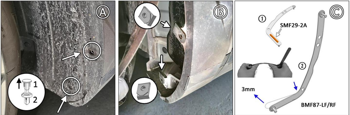
**FIGURE D/E** Position BMF87-LF/RF bracket behind mud flap. Place logo-side of mud flap facing rear of the vehicle against mounting points on liner and bracket. Use 1.5SS & SMWASH to fasten points 2 & 4. Use SSLNUT & SMWASH for mounting points 1 & 3. Ensure inner foam spacer contacts liner. Repeat Figure C as needed.
