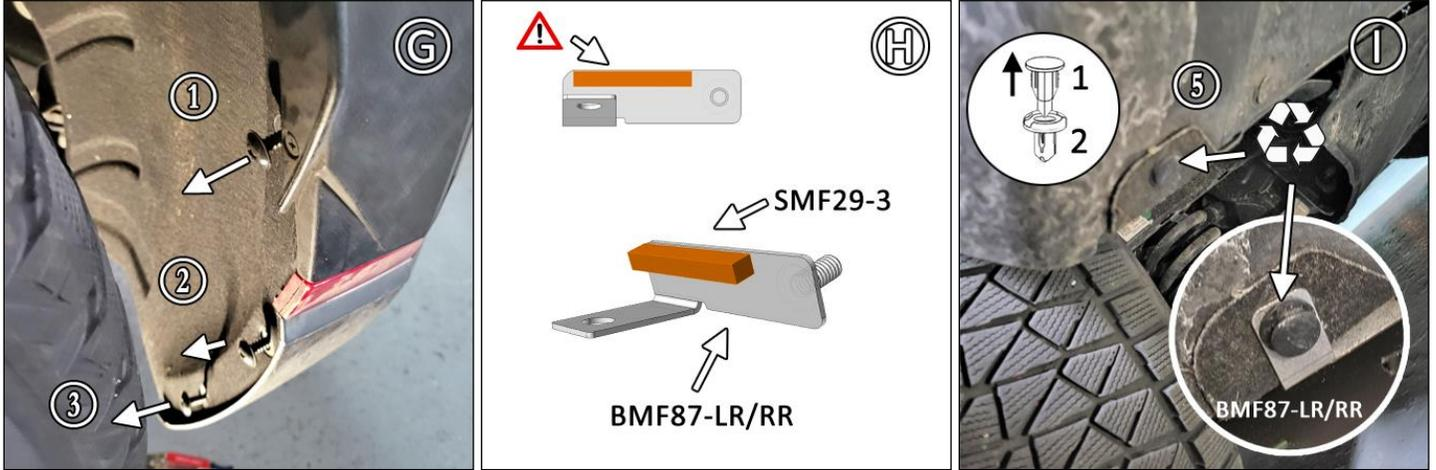
**FIGURE J** Place logo-side of mud flap facing rear of the vehicle against corresponding mounting points. Use 1.5SS & SMWASH to fasten points 1 - 3. Use SSLNUT and SMWASH for mount #4. Do not fully tighten.
